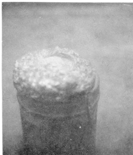
FIGURE 5. Metal Button Showing Imprint of Stir Blade
