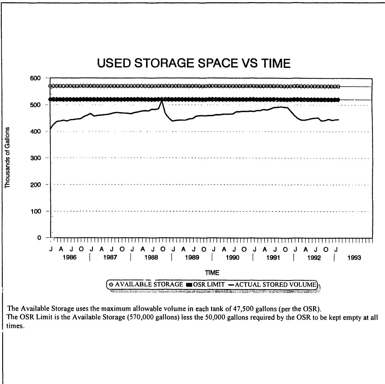
Figure 6. Used storage space versus time. (ORNL-DWG. 93-5637)
