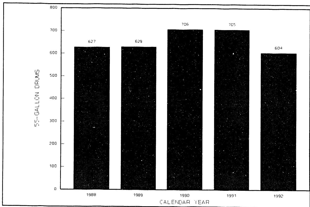
Figure 2. Sludge generation at the PWTP. (ORNL-DWG. 93-5633)
