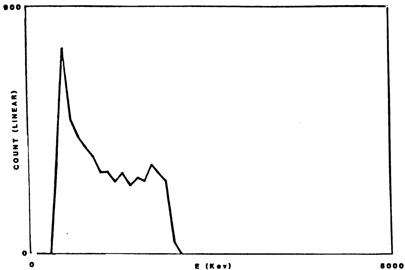
Fig. (5-5): A typical energy spectrum of recoil protons for interactions of 800 MeV protons with hydrogen gas in time-of-flight setup.
