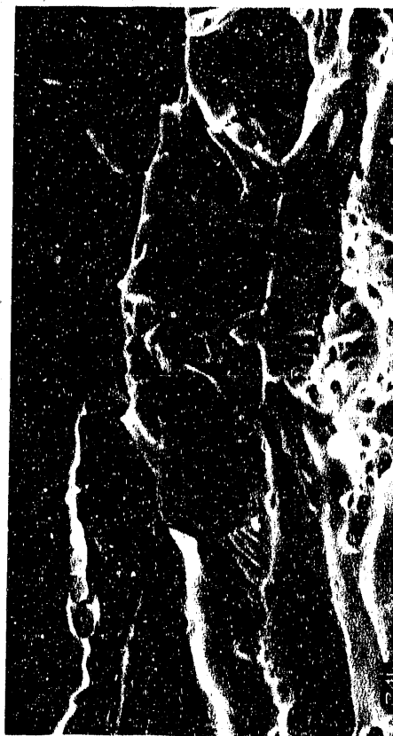
Fig. 60. Fracture surfaces at a higher magnification of room-temperature tensile-tested specimens of iron-aluminide alloy [FAL (Heat 13008)]. (a) Stress relieved and annealed for 1 h at 700°C, and both were followed by air cooling; (b) stress relieved and annealed for 1 h at 750°C and 700°C, respectively, and both were followed by oil quenching; and (c) stress relieved and annealed for 1 h at 750°C, and both were followed by oil quenching. Source: INEL/EG&G.
