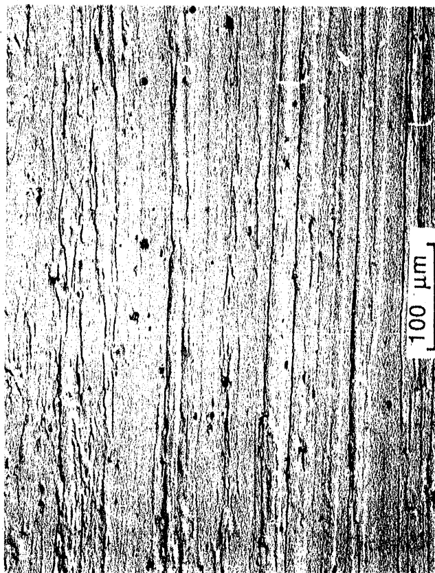
Fig. 50. Optical microstructure of iron-aluminide specimen [FAL (Heat 13008)] with a stress relief of 700°C for 1 h followed by oil quenching. No annealing treatment was given to this specimen.
