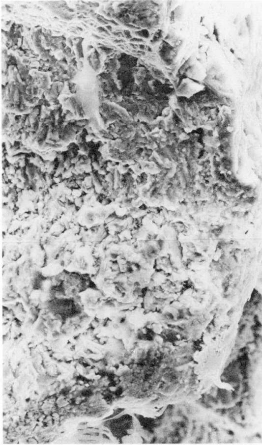
a. UPPER CRACK BRANCH, STRESS CORROSION FRACTURE
