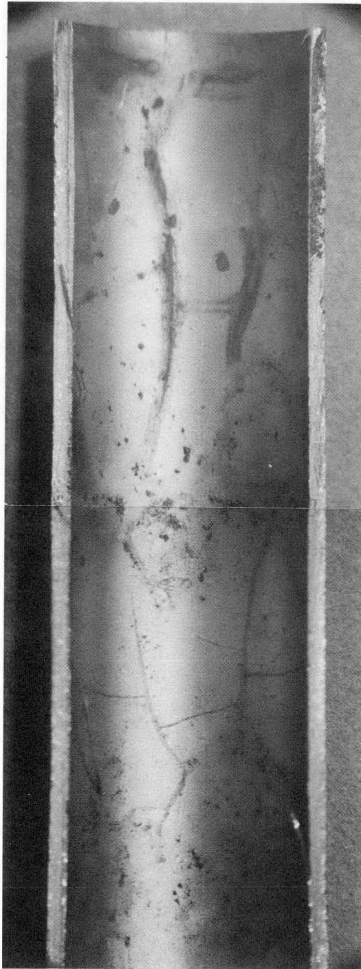
Figure 3.2-10 Macrophotographs Of One-Half Of Inside Surface Of Cladding Section 3 From Rod KE-2225 ~ 3.5X
