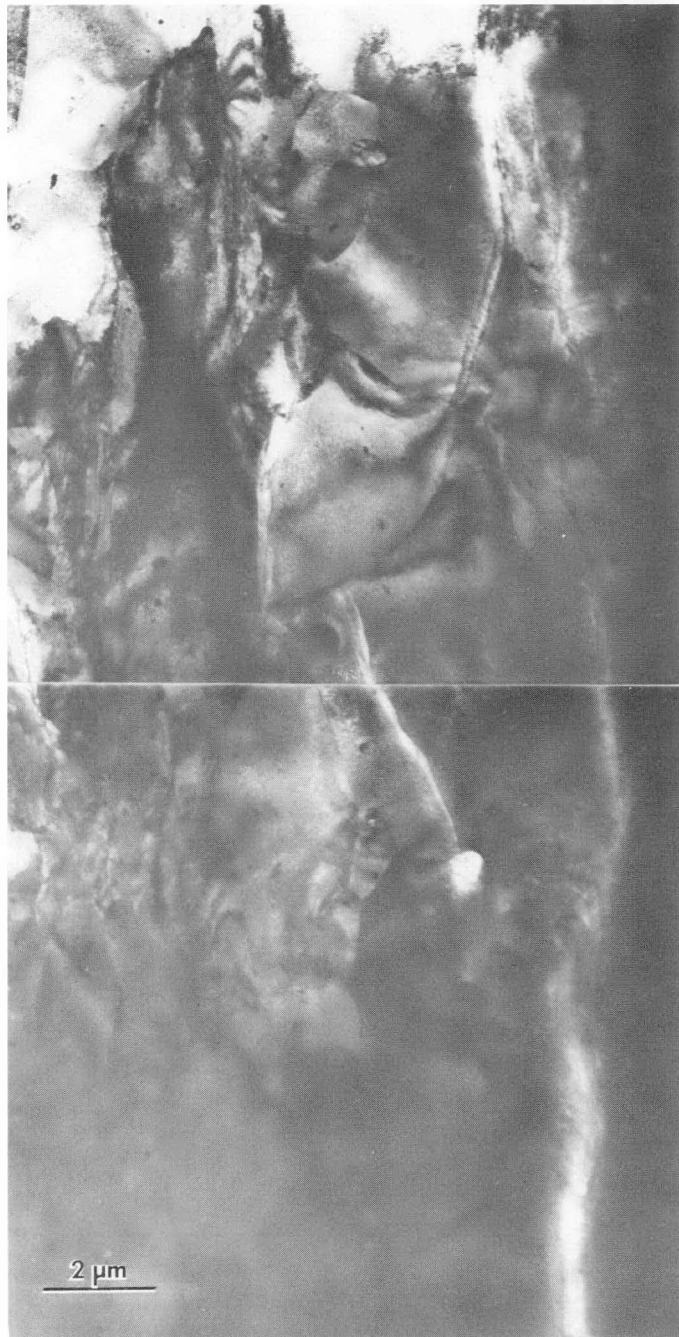
Figure 3.2-66. Continuous Grain-to-Grain Features in Fuel Rod KE-2225
