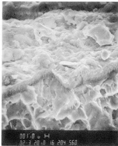
Figure 3.3-37 Surface Oxide of Specimen 14K
