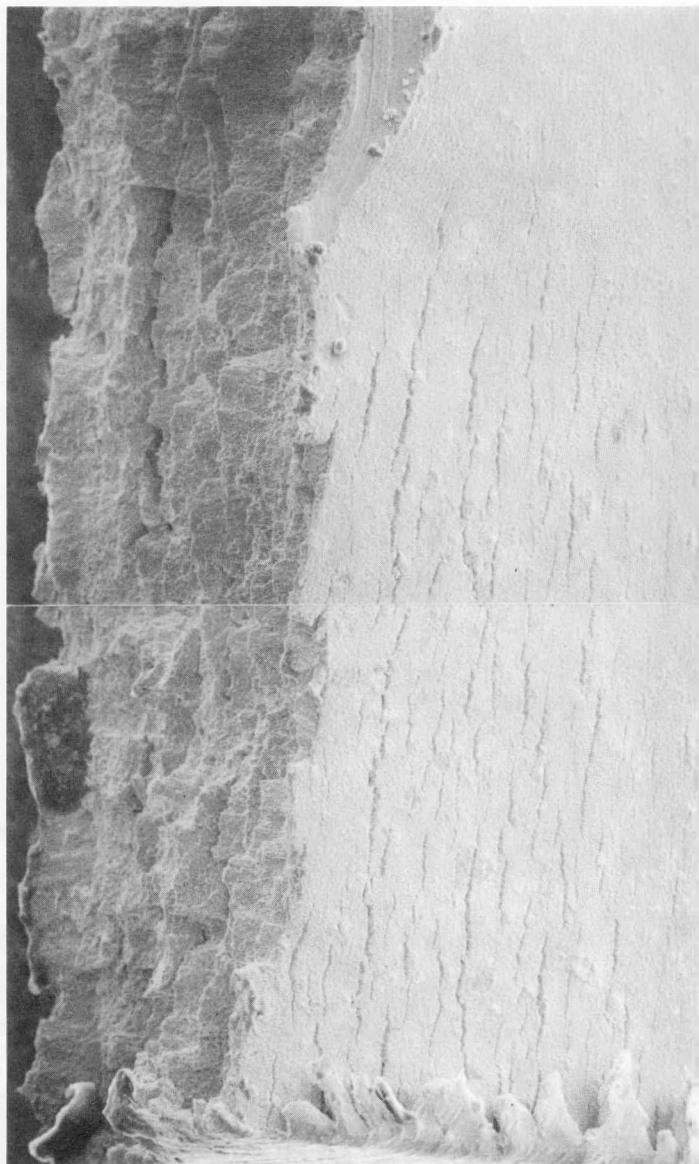
a. CRACK SURFACE AND INSIDE CLADDING SURFACE 100X
