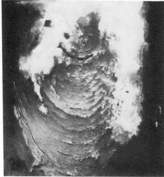
Figure 3.3-25 Circular Cracks Near Large Uranium Containing Deposit on Inner Surface of Specimen 2K (Area B, Fig. 3.3-23) 30X Neg. No. MSD-204129
