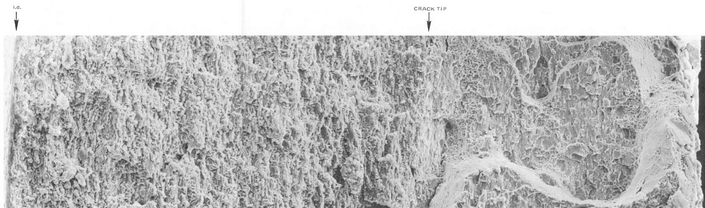
Figure 3.2-21. Rod KE-2225, Crack A; Area of Part-Through Crack Penetration (See Figure 3.2-16 for Location) ~ 400X
