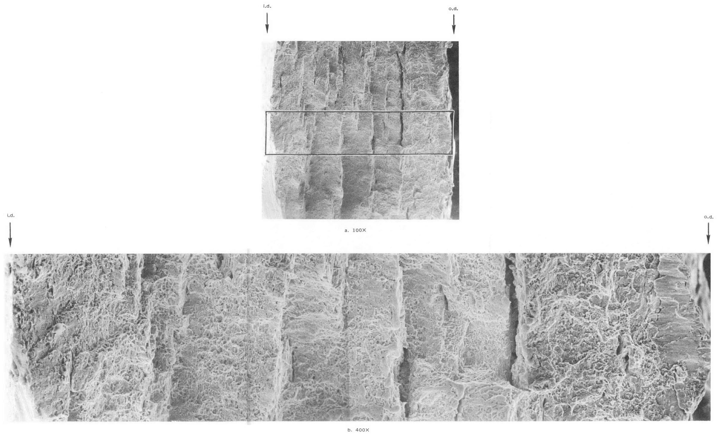
Figure 3.2-33. Rod KE-2225, Section 5C; Ductile Fracture Surface
