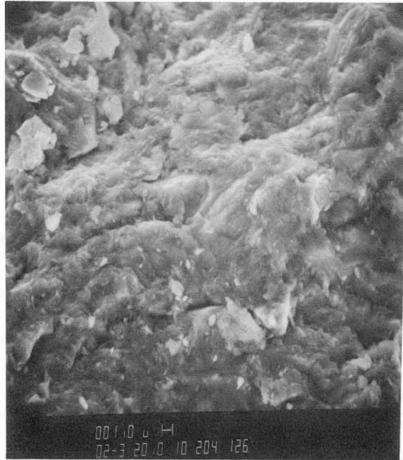
Figure 3.3-29 Fracture Surface of Defect from Specimen 2K
