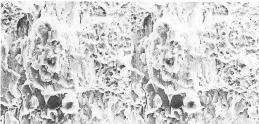
c. QUASI-CLEAVAGE AND DIMPLES
