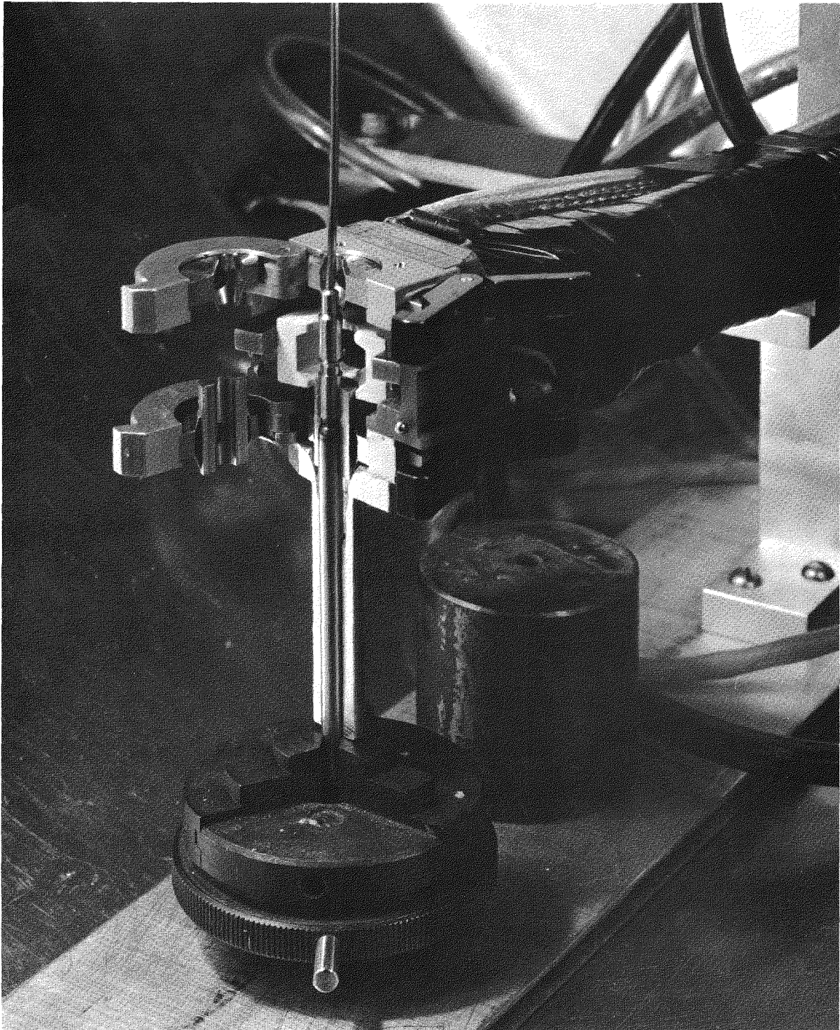
Fig. 20. Fuel-element and Thermocouple Preassemblies Positioned in Welding Head. ANL Neg. No. 104-77-105.
