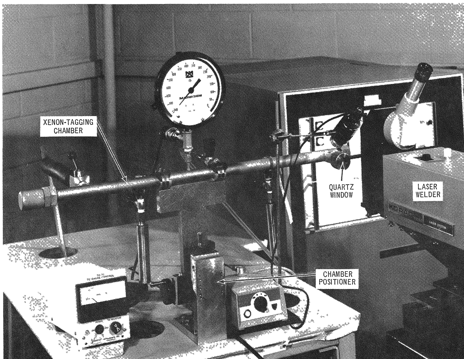
Fig. 21. Apparatus for Xenon-tagging Fuel Elements for XX08. ANL Neg. No. 104-76-299.
