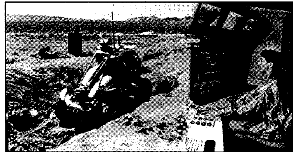
Figure 4. The REmote TeleRobotic Vehicle for Intelligent Remediation (RETRVIR) is shown depositing an uncharacterized object from Sandia's explosive test site with the operator's graphical planning and programming interface shown on the right.
