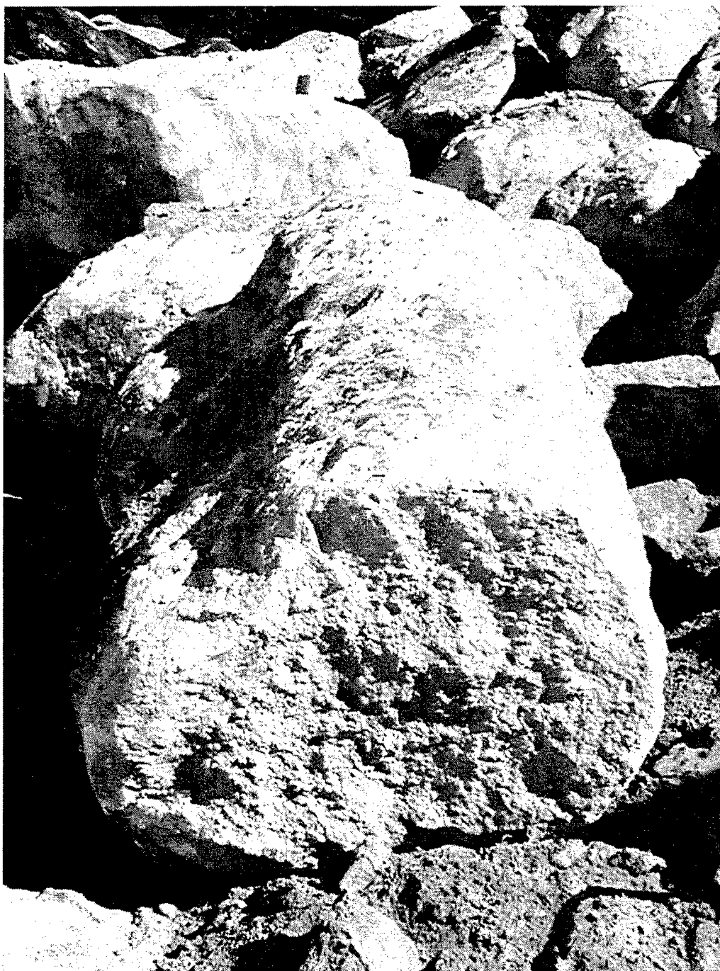
Figure 7.27 Section of the cement layer of the BNL close-coupled barrier showing adjacent columns.
