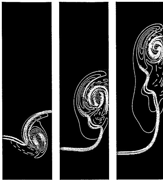
**Figure 1.** Evolution of the heat release rate (color) and vorticity fields (contours) for the stoichiometric flame, for a time span of 1 ms. Frames are at 0.2, 0.6, and 1.0 ms. Solid/dashed contours denote positive/negative vorticity.
