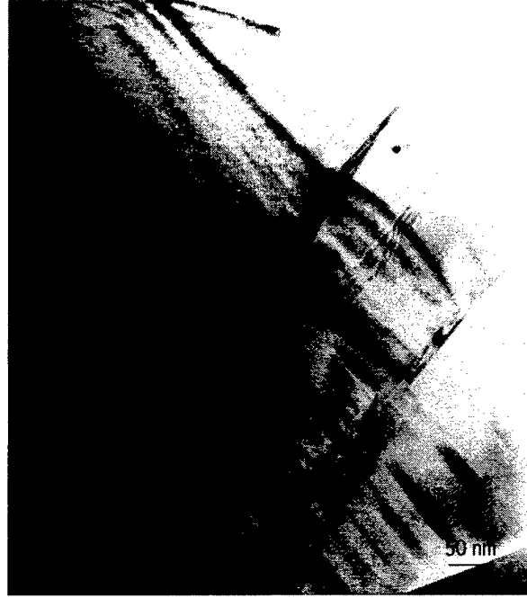
Figure 22 TEM of stacking faults. Twins and a grain boundary are also shown.
