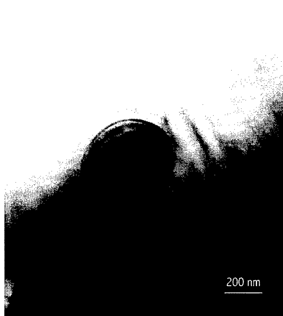
Figure 20 TEM shows the spherical Gd 2 11 phase.
