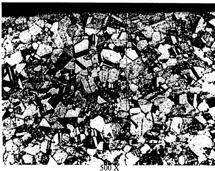
Figure 2. SURV-5 Inconel X750. No significant change in structure is apparent. ( \text{HNO}_3 + Acetic + \text{H}_2\text{O} etchant)
