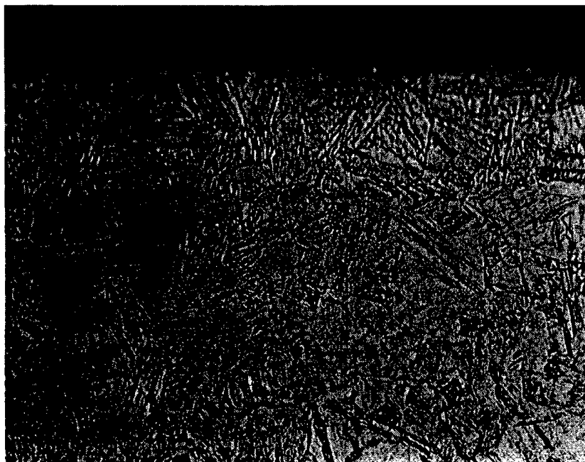
Control Sample Type 17-4 PH ( \text{FeCl}_3 + HCl etchant)
