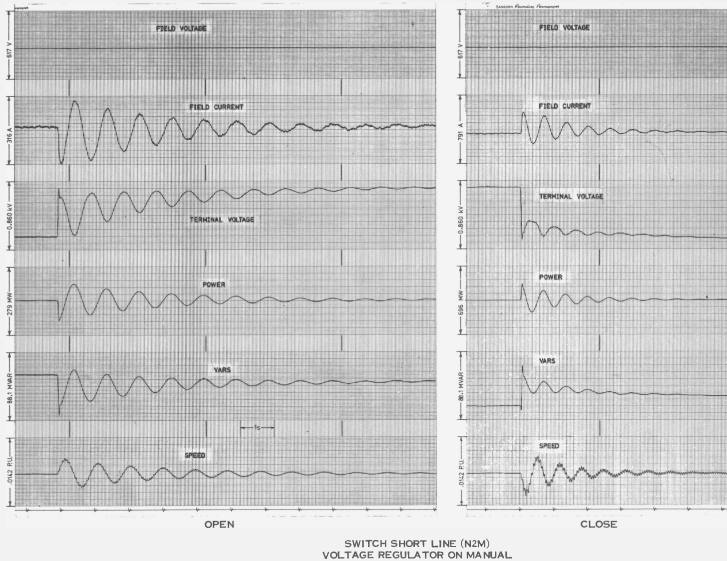
Figure 3-9. Nanticoke Line Switching Test 4, Oscillograms of Generator Variables.
