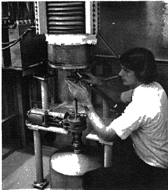
Fig. 2-22. Lower section of 0.20-m primary burner system including susceptor, induction coil and capacitors, gas distribution, product can, and plenum drain can
