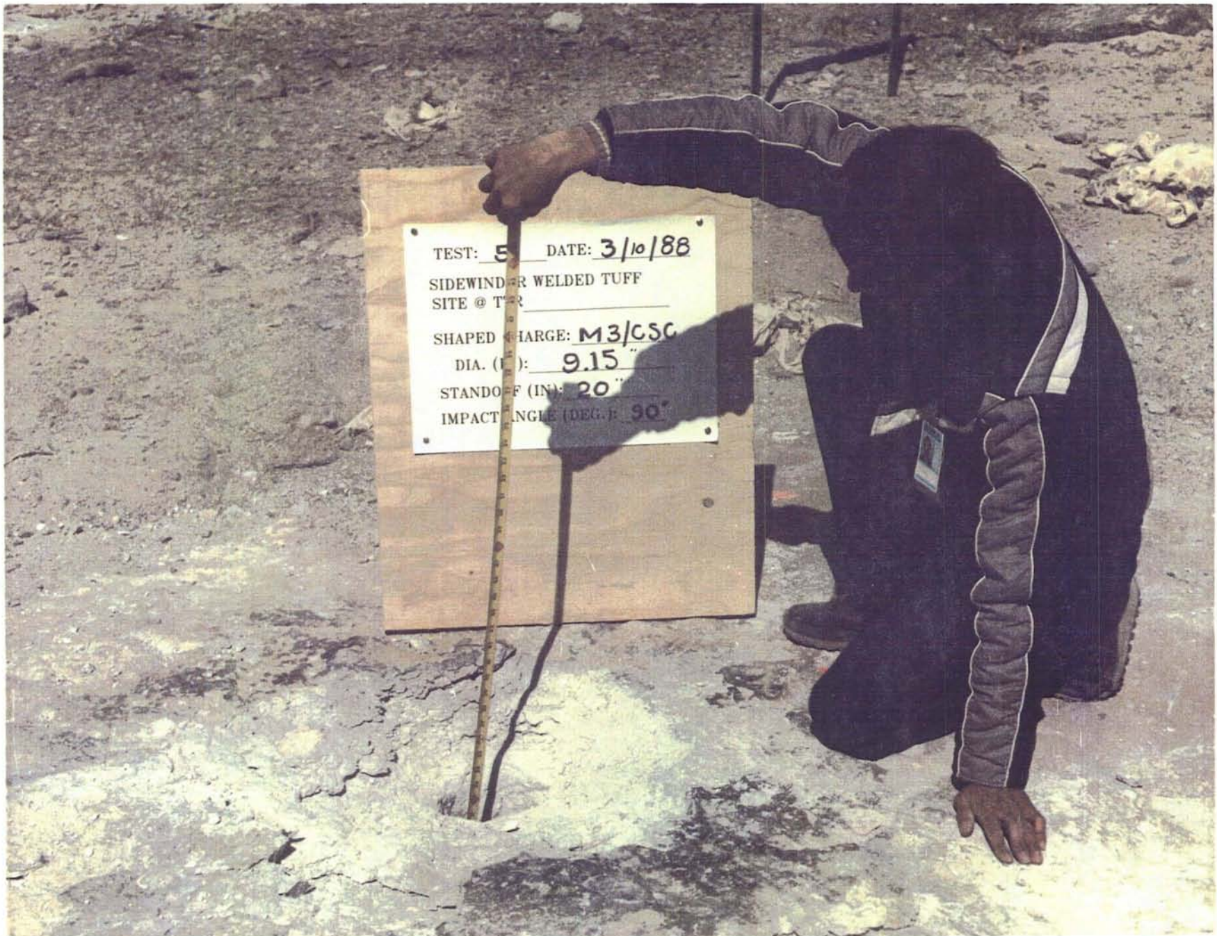
Figure 7. Steel Tape Used to Measure Hole Depth
