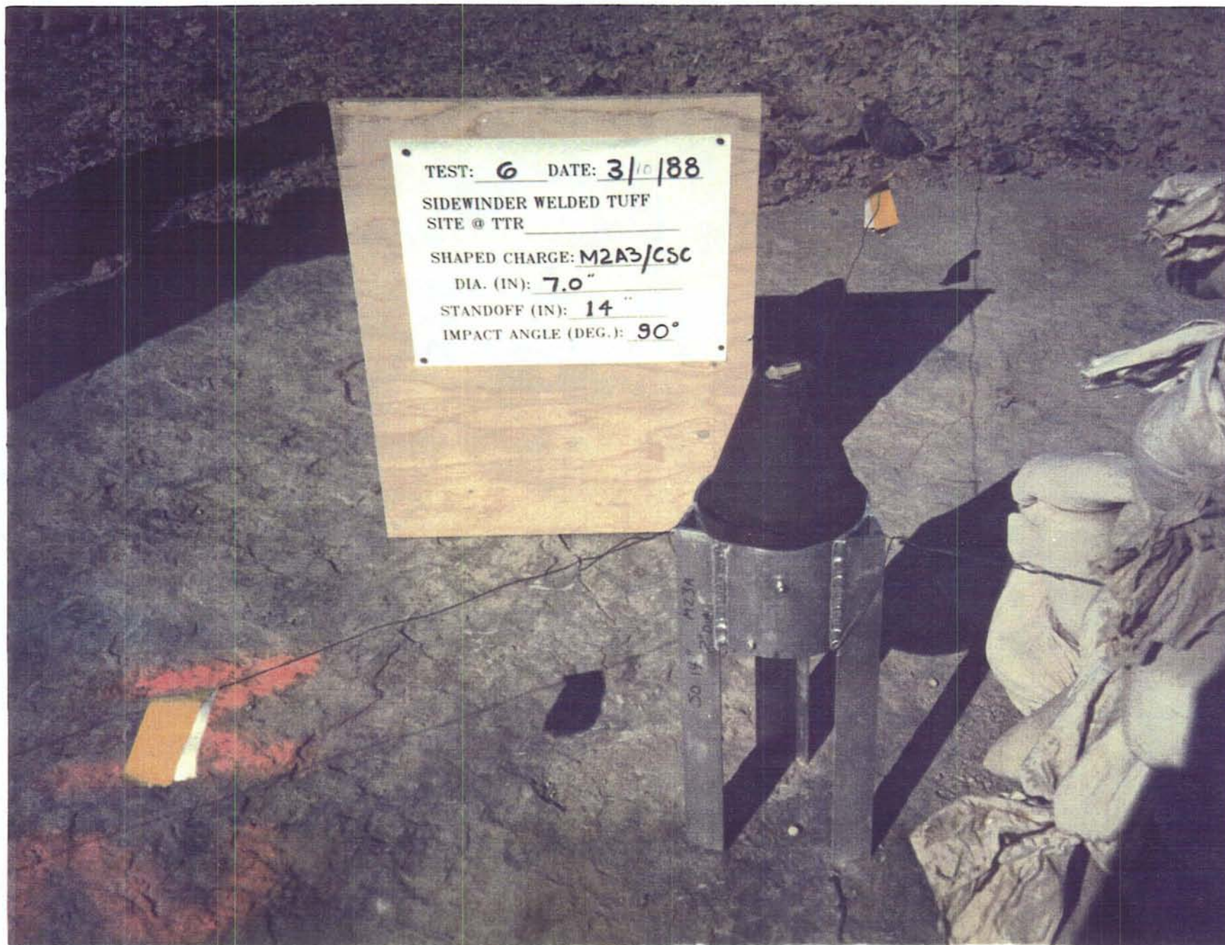
Figure 32. 7.0 Inch Diameter CSC Test Configuration
