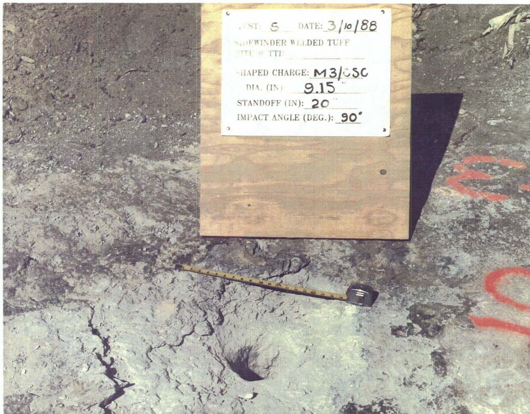
Figure 35. 9.125 Inch Diameter CSC Generated Hole in Tuff
