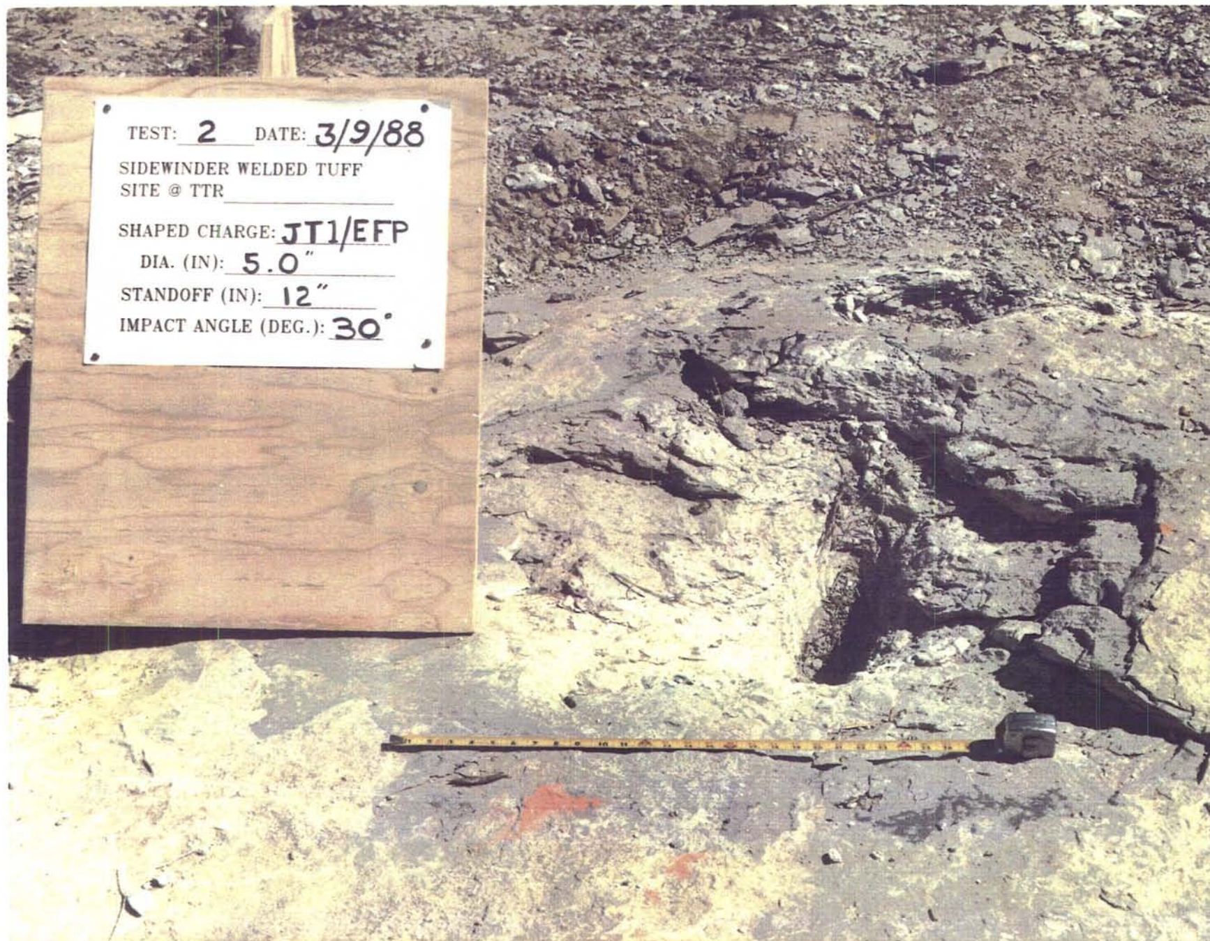
Figure 45. EFP Slug Generated Hole in Tuff Target
