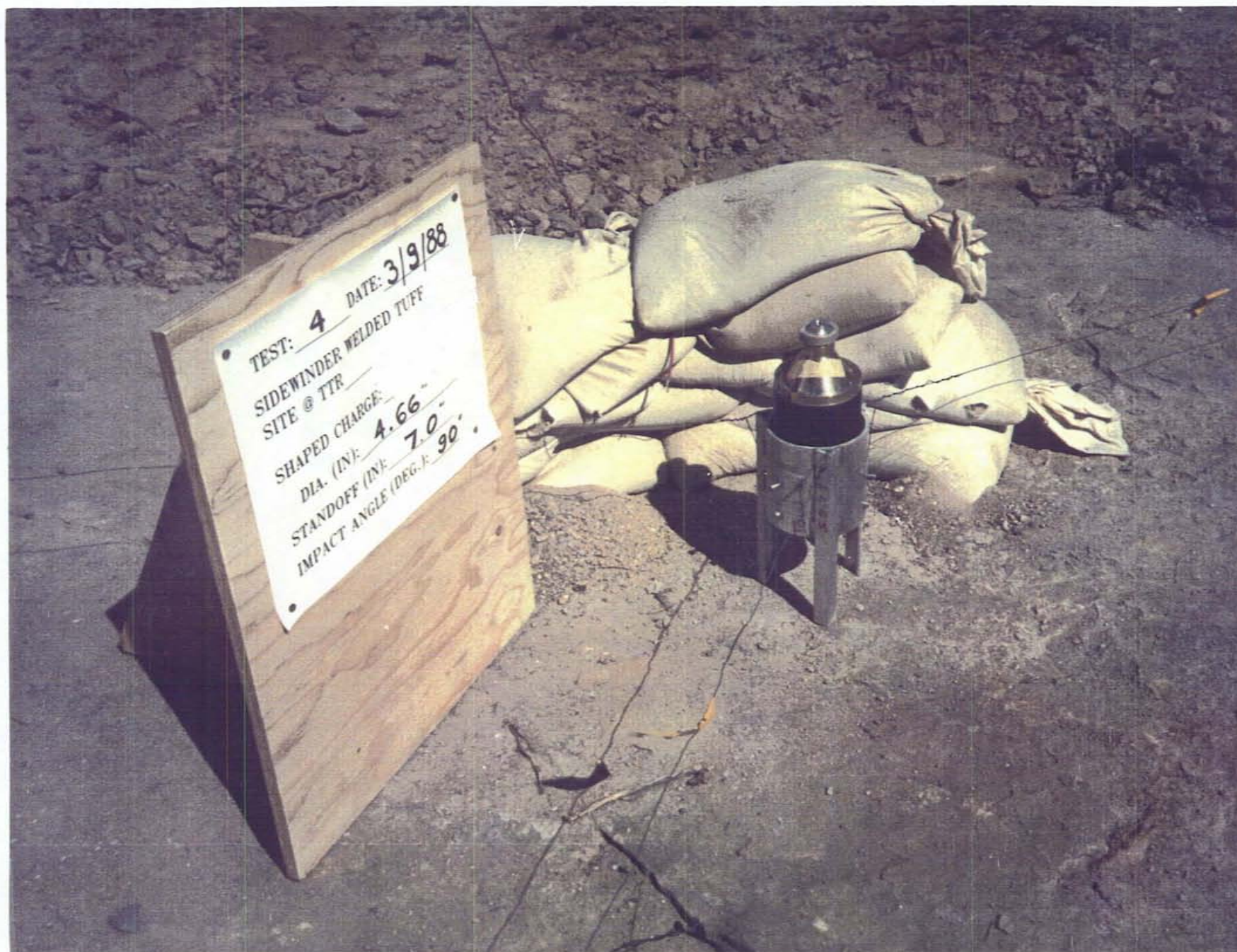
Figure 30. 4.66 Inch Diameter CSC Test Configuration
