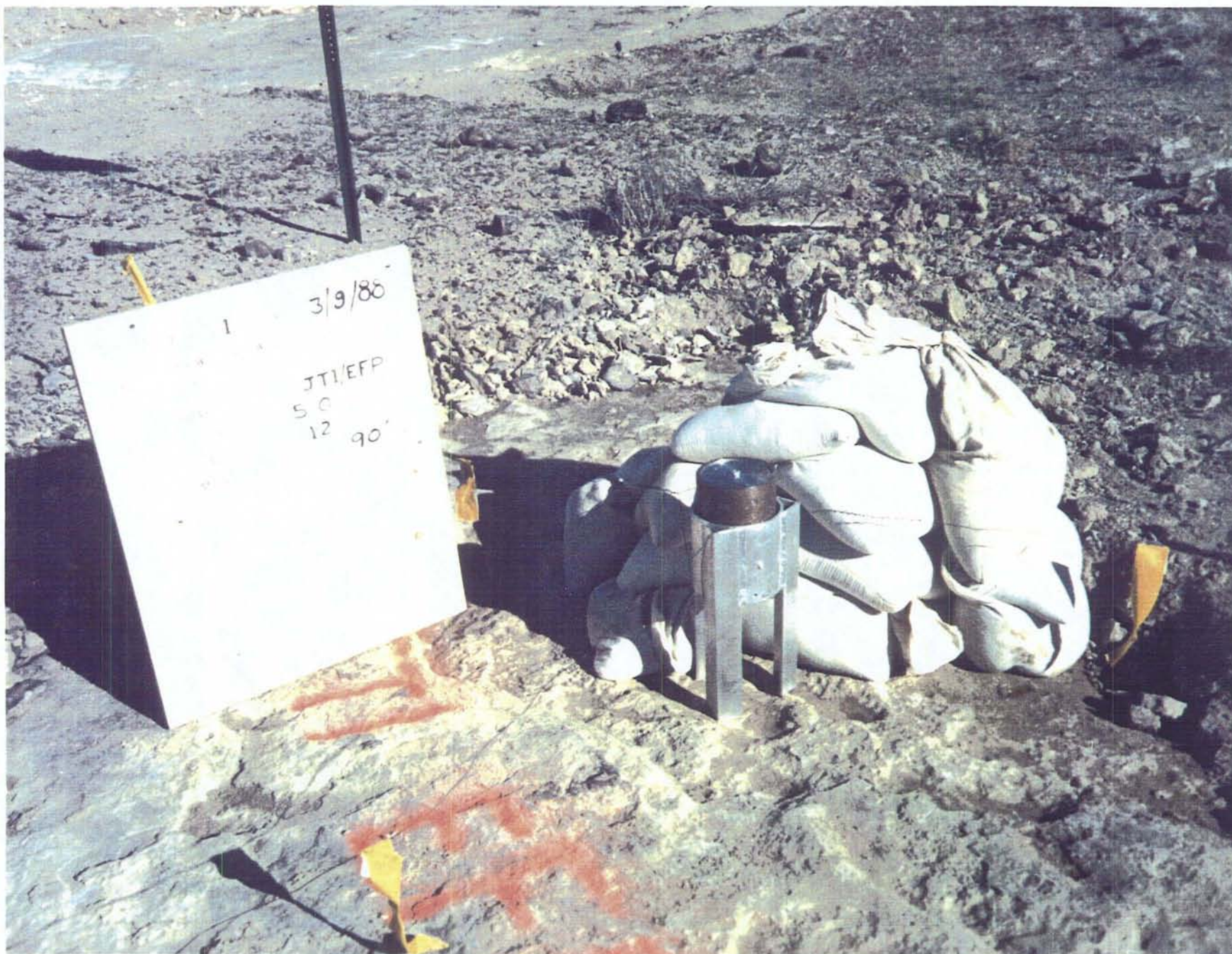
Figure 42. EFP Test Configuration for 90 Degree Impact of Tuff Target
