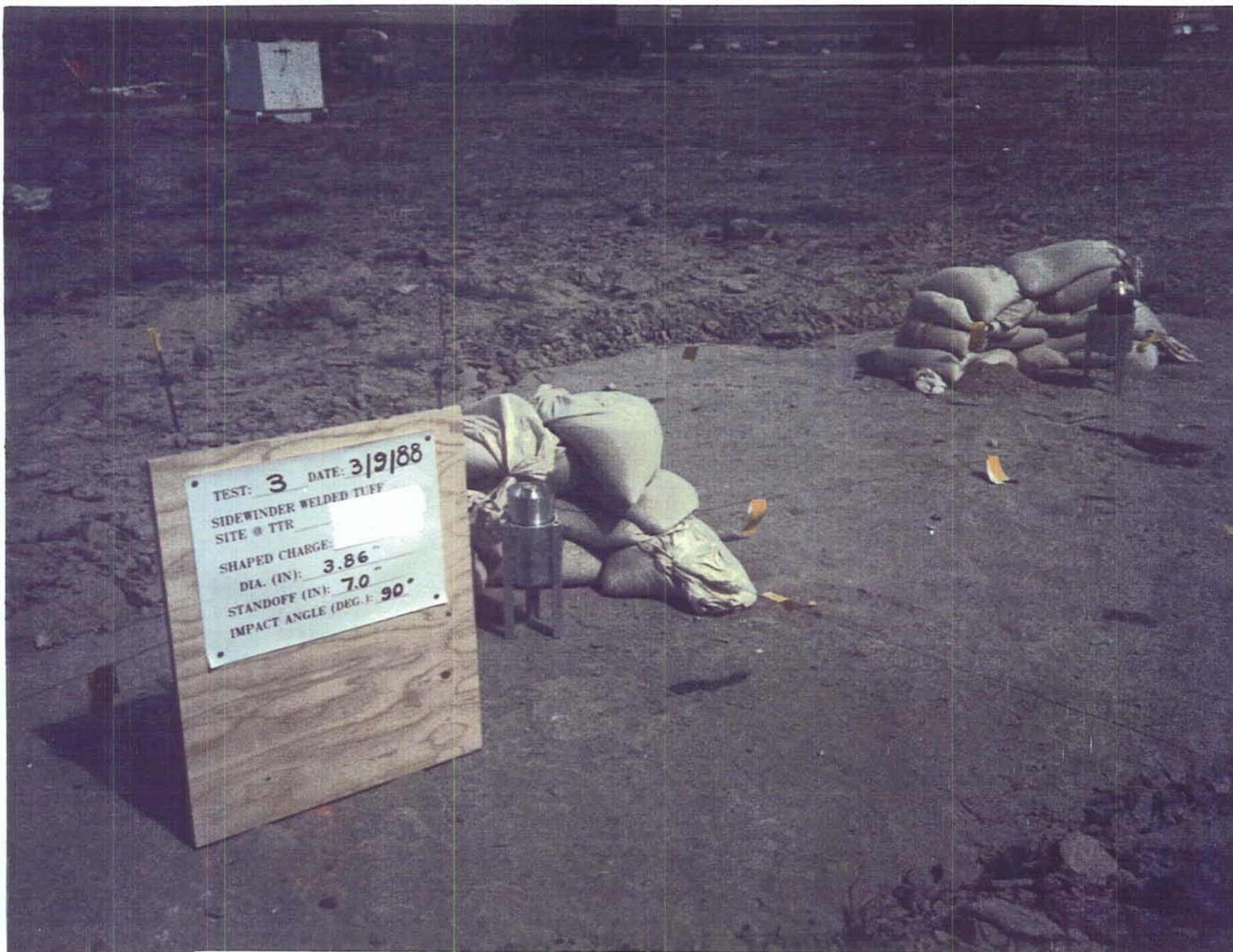
Figure 28. 3.86 Inch Diameter CSC Test Configuration
