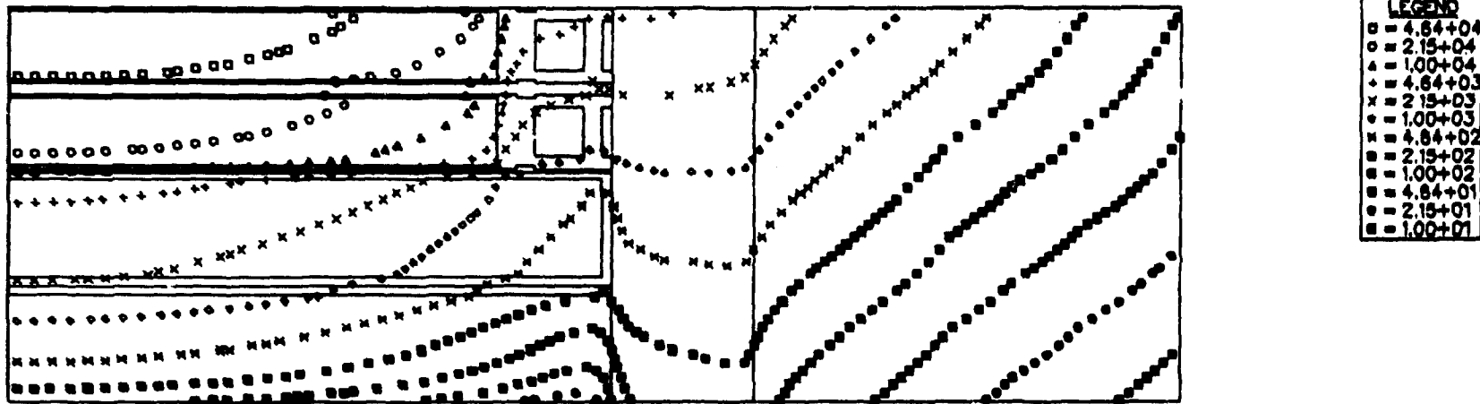
Fig. 30. Isoplot contours for the gamma-ray flux above 1 MeV within the UO 2 blanket + reference inner shield configuration (Configuration II.B).
