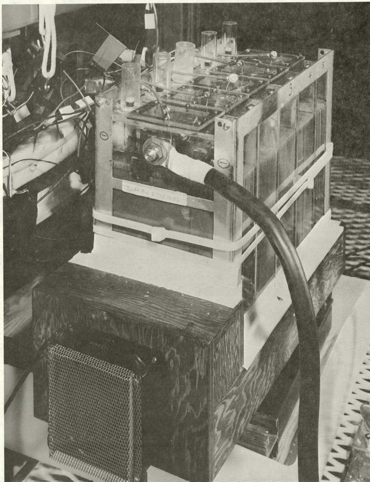
Fig. III-2. An Eagle-Picher Nickel/Iron Module with Forced Air Cooling Under Test at NBTL. ANL Neg. No. 308-80-29K.
