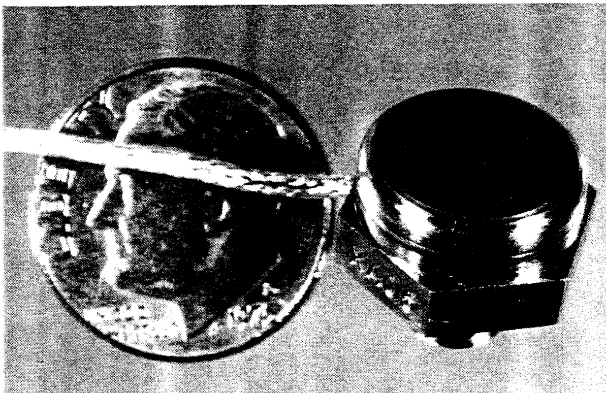
Figure 3. Rugged, Undamped Piezoresistive Accelerometer
