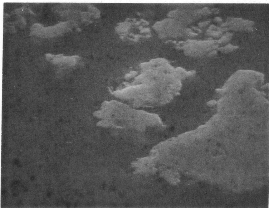
Fig. 12a. SEM of an area rich in Ca, Fe, and Si. 5000X
