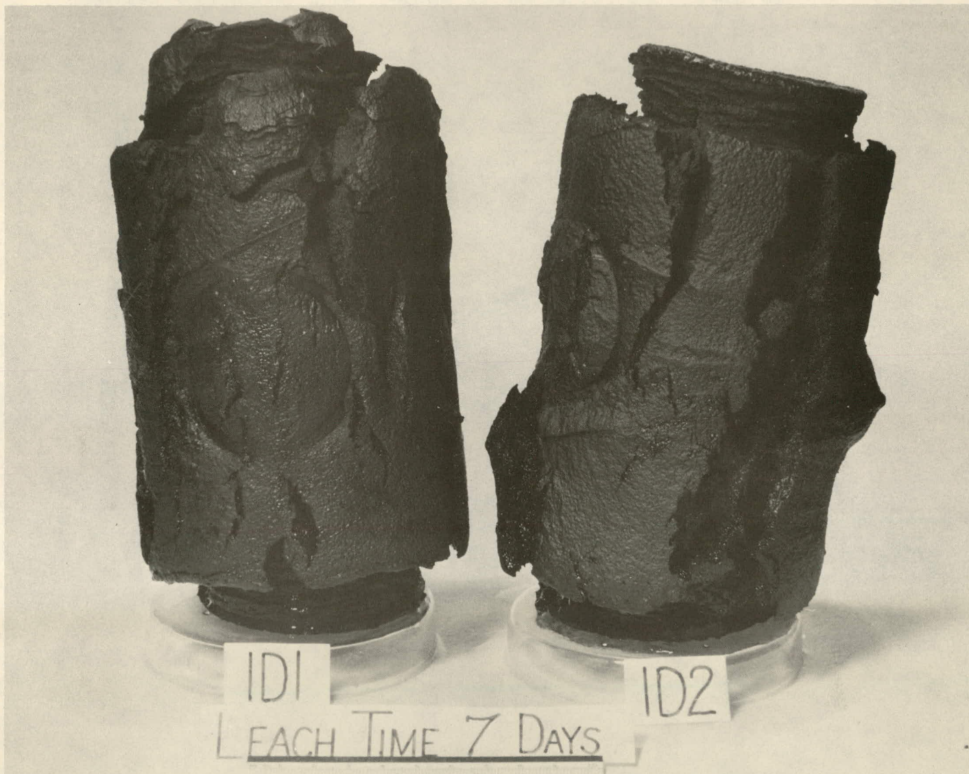
Figure 6. Bitumen Waste Form ID2 (41.4 Wt.% \text{Na}_2\text{SO}_4 ) after Seven Days of Leaching in Distilled Water.
