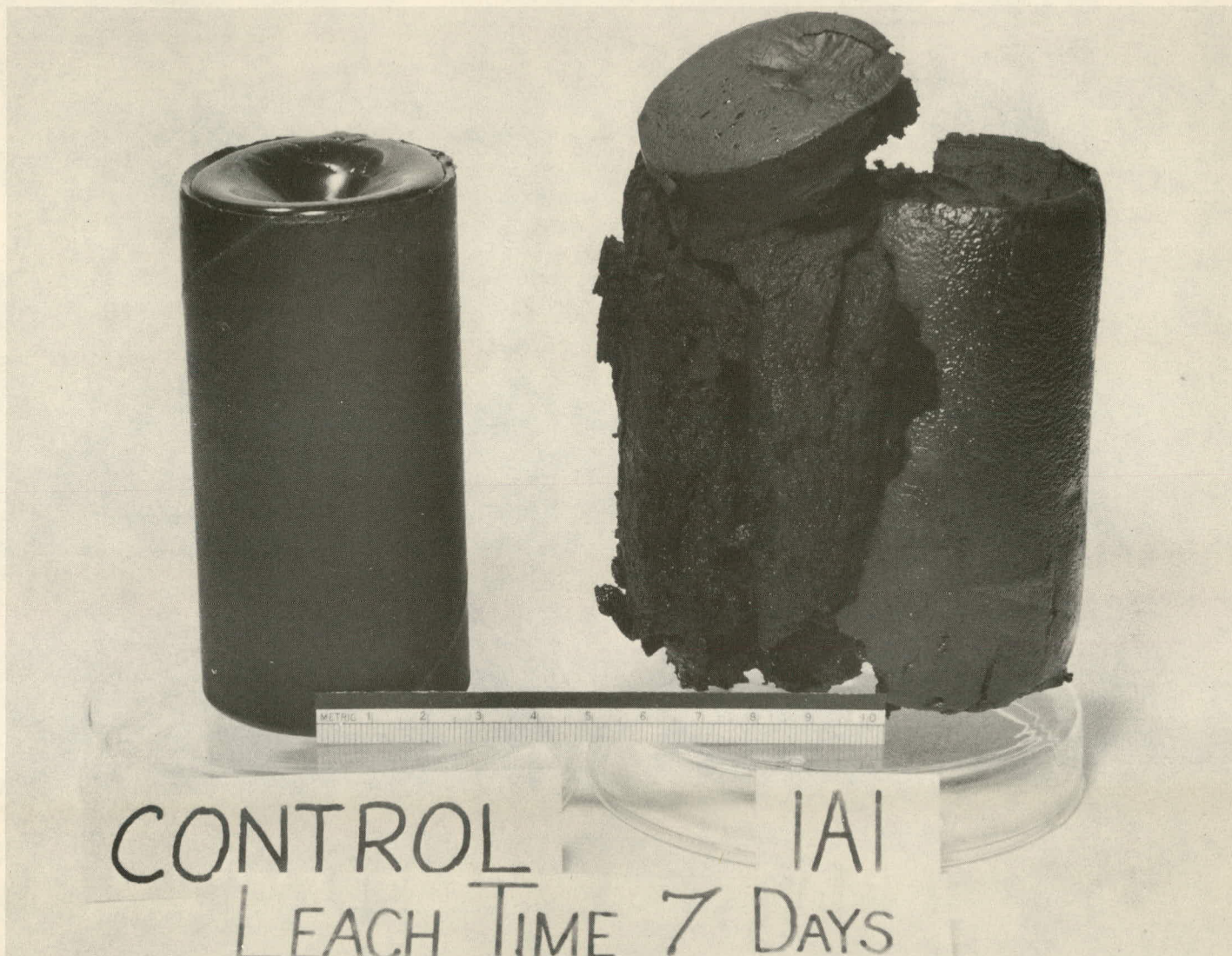
Figure 4. Bitumen Waste Form 1A1 (28.5 Wt.% \text{Na}_2\text{SO}_4 ) after Seven Days of Leaching in Distilled Water.
