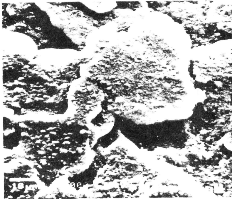
Figure 18. SEM of F6331/SR-125/2468 Aluminum Flake Coating
