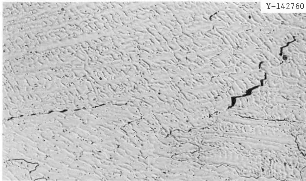
Fig. 17. Example of Scattered Cracks or Voids That Were Observed in As-Welded ERNiCr-3. Etched with 5:1 HCl:HNO 3 . 200×
