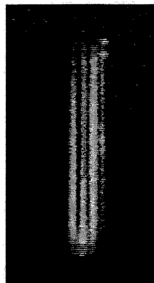
Figure 4.11. An image of four filaments across a 1.5 cm long GaAs PCSS was produced with 4 line-triggers. Precise control of the filament location and shape was achieved as these filaments carry 100-150 A each and are less than 1 mm apart.
