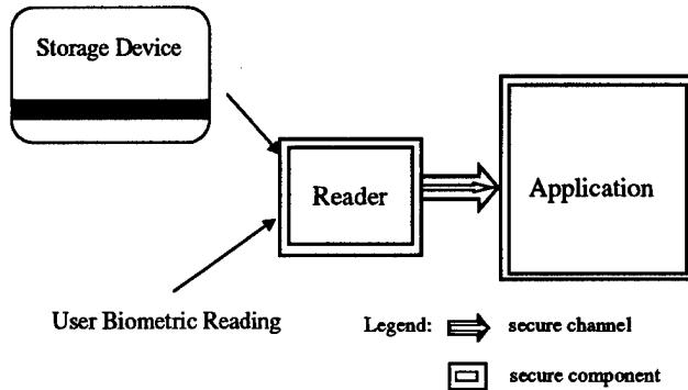
Figure 2: Secure application with biometric authorization
