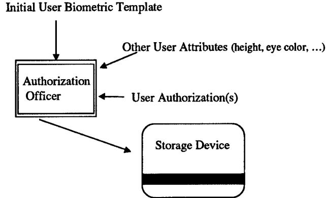
Figure 1: Storage device initialization
