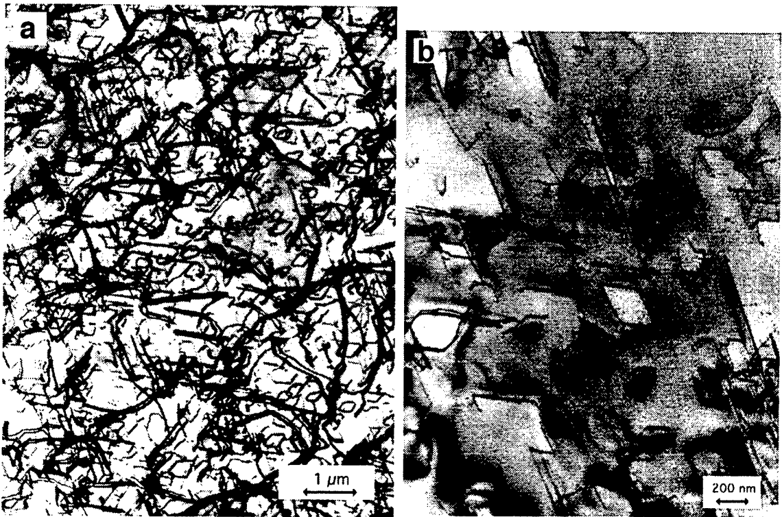
Fig. 7. TEM microstructure of FA-180 (1150°C/oil quenched) specimen creep tested at 593°C/207 MPa for 6480 h without rupture (gage section), showing (a) creep-induced dislocation network structure together with a dense dispersion of dislocation loops, and (b) higher magnification showing several individual loops containing kinks and jogs, present on orthogonal habit planes ( g=011[B2] ).
