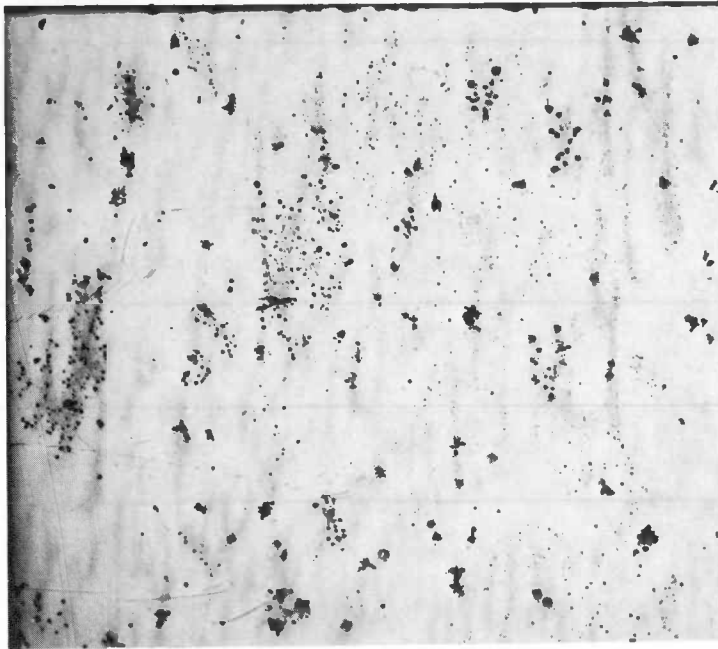
FIG. 76 - Cored Structure in Buck 6. STBS Etch. Mag. 6X
