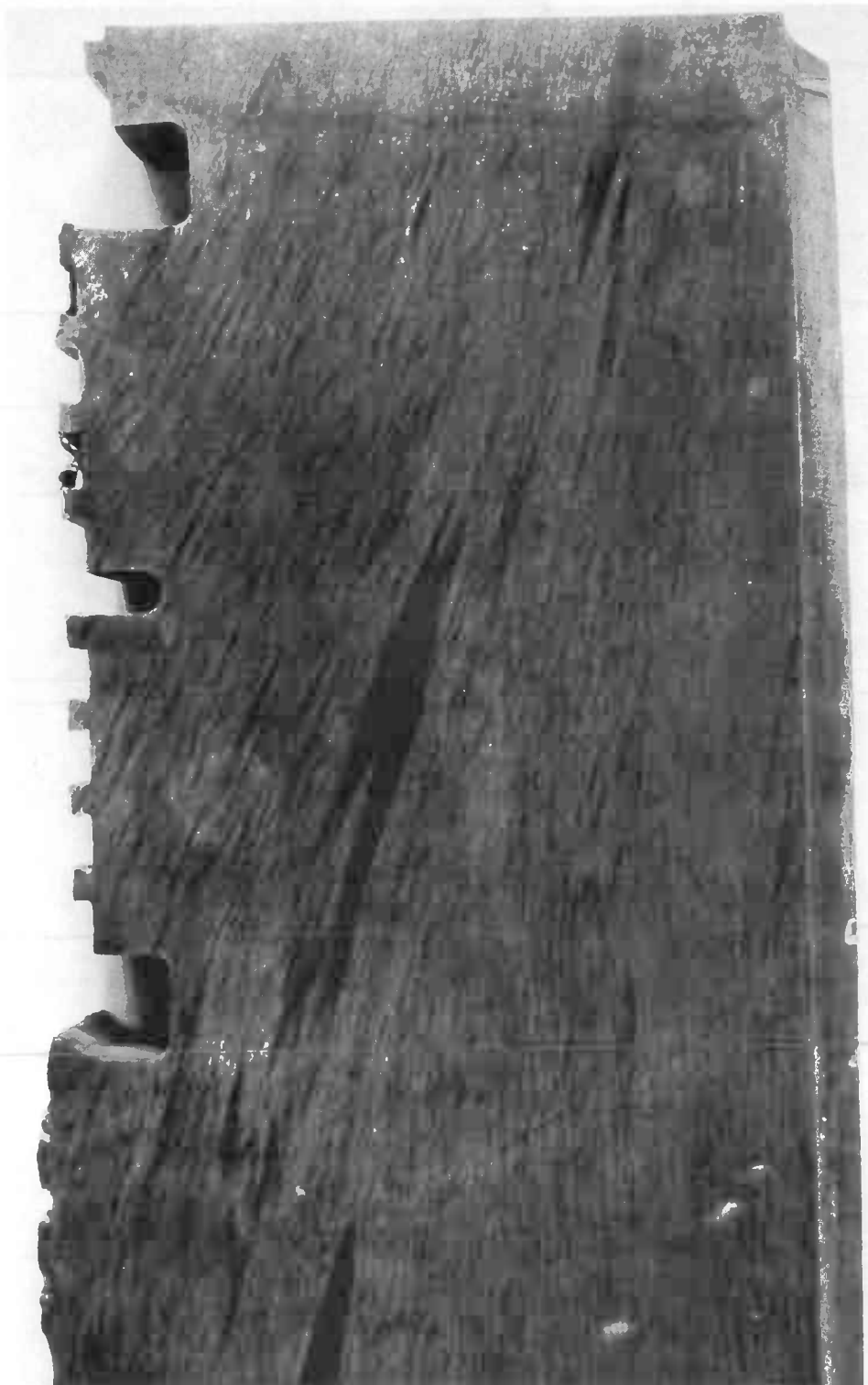
Fig. 2.2— 2.5X Ammonium persulfate macroetch showing segregation pattern in the Gallatin forging
