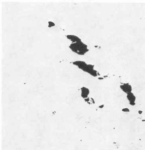
FIG. 30 - Large Flaw from Joppa 3 Piece J7A1-6. Material Removed from 332° Plane of Polish is Indicated. Mag. 6X
