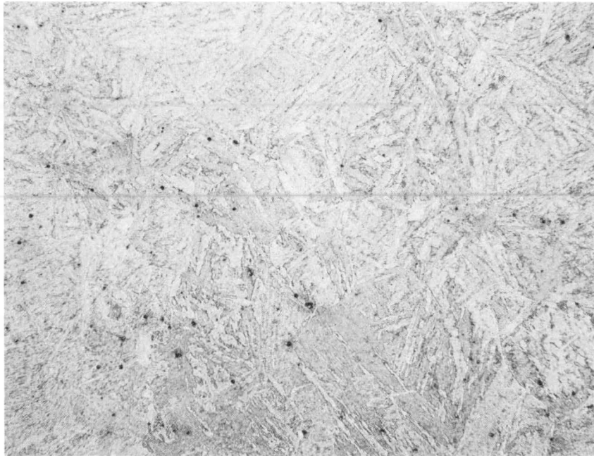
FIG. 77 - General Microstructure of Buck 6. 2% Picral Etch. Mag. 100X
