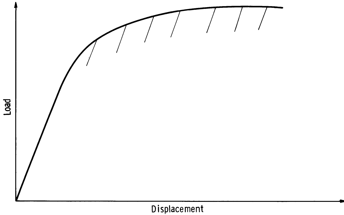
Fig. 4.9 – Schematic representation of the unloading compliance technique for J resistance curve determination
