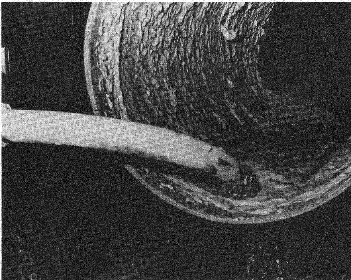
FIGURE 1. - Flocculated clay waste discharged from mixer through pipe into rotating screen.
