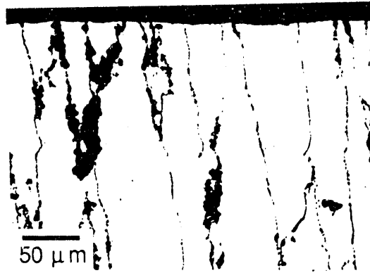
Fig. 3. Polished cross section of \text{Ni}_3\text{Al-10\% HfO}_2 exposed to dry air at 800^\circ\text{C} for 171 h.
