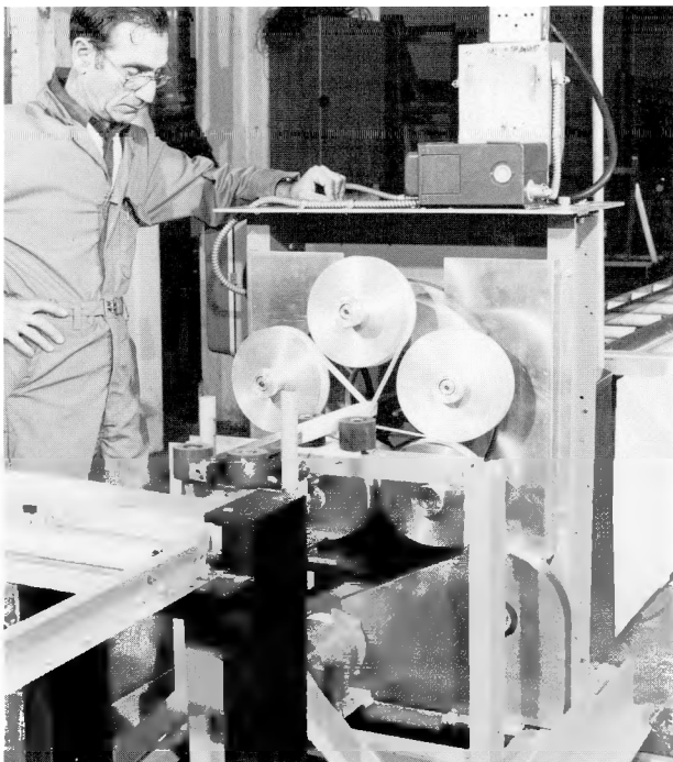
Figure 60. 5-Head automatic taping machine—Large Coil Program.
