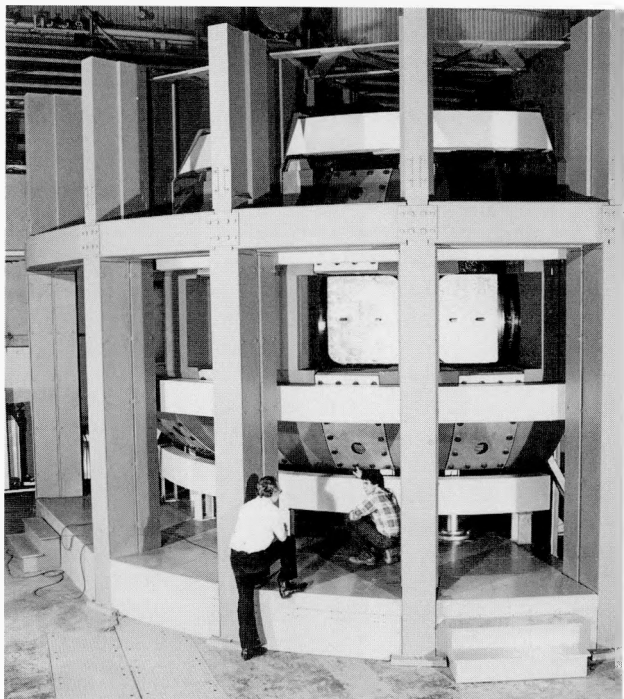
Figure 50. PF coils in position on M-3 Mockup.
