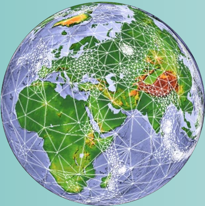
Visualization tools assist analysts in interacting with the resources of the Knowledge Base. For example, a display of the tessellated globe shows the points (intersections of lines) where corrections for path effects are stored.
