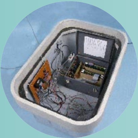
In the DOE prototype infrasound system, each array of sensors is solar-powered and has a meteorological system (top). Each sensor with accompanying noise-suppression hoses is installed on top of a buried tamper-proof enclosure (center) containing the data-acquisition system and transmitter/receiver (bottom).
