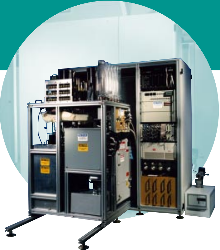
The Automated Radioxenon Sampler/Analyzer performs ultra-sensitive analysis of four xenon isotopic gases in near real time. The xenon is collected on a charcoal sorption bed and is then thermally desorbed, purified, and measured by gamma-ray spectrometry. The gamma-ray spectra and radionuclide concentrations are transmitted to data centers. The gas samples can be retained for laboratory confirmatory analysis.
