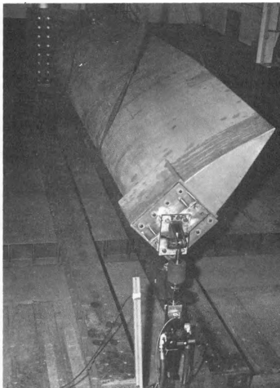
Figure 5. - Twenty foot long laminated wood wind turbine blade test specimen.
