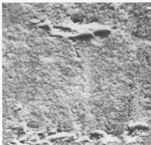
Figure E-32. Scanning Electron Micrograph of the Crevice Region Near the Top of Specimen H-7E-4-1 Showing the Five Locations at which Higher Magnification SEM and EDS Analyses were Obtained (50X)*
