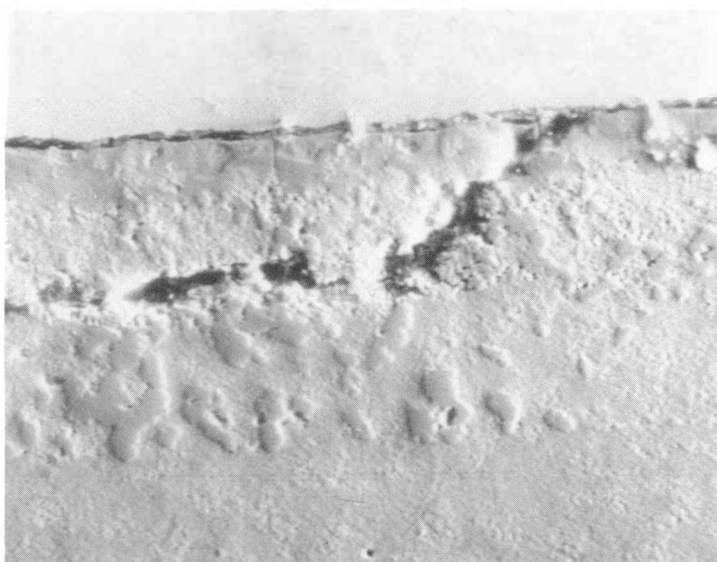
Figure B-27. SEM of the Steel/Oxide Interface, Showing Crack/Crevice - Sample AA-8.
