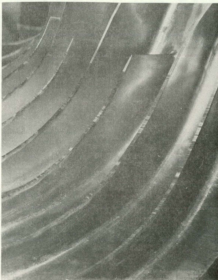
Figure VI-10. Impeller Tip Damage Due to Interference Rub
