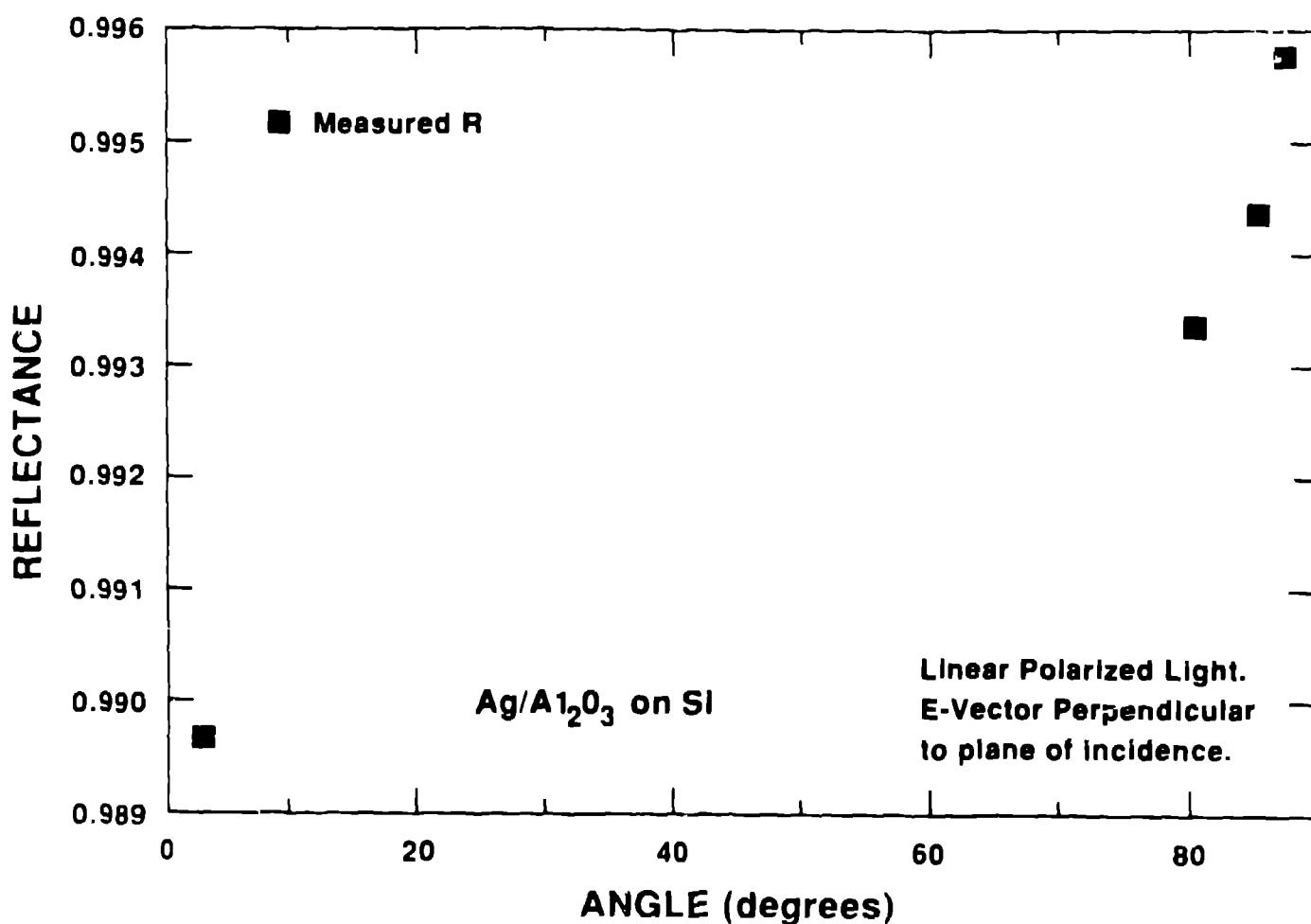
Figure 4. Measured reflectance of a protected silver reflector at various angles.
