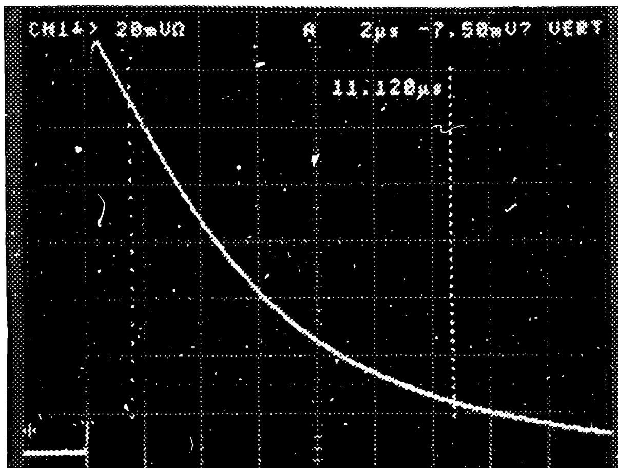
Figure 3. Oscilloscope output showing cavity decay time ( $11.120 \mu\text{s} = 2\tau_C$ ).
