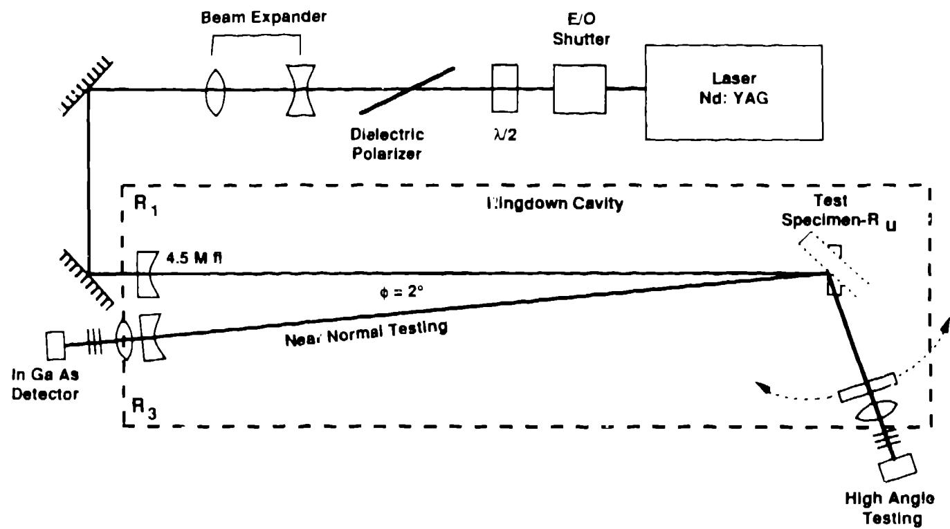
Figure 1. Schematic of the ringdown reflectometer system.
