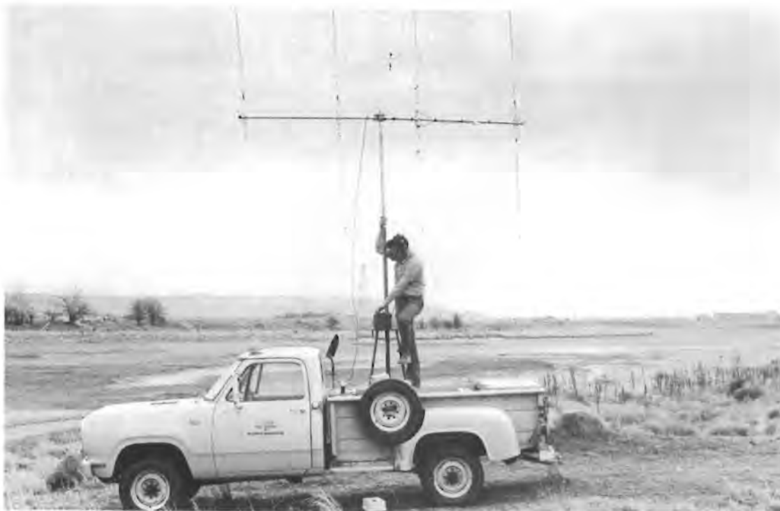
FIGURE 3. Truck with mounted receiving antenna.
