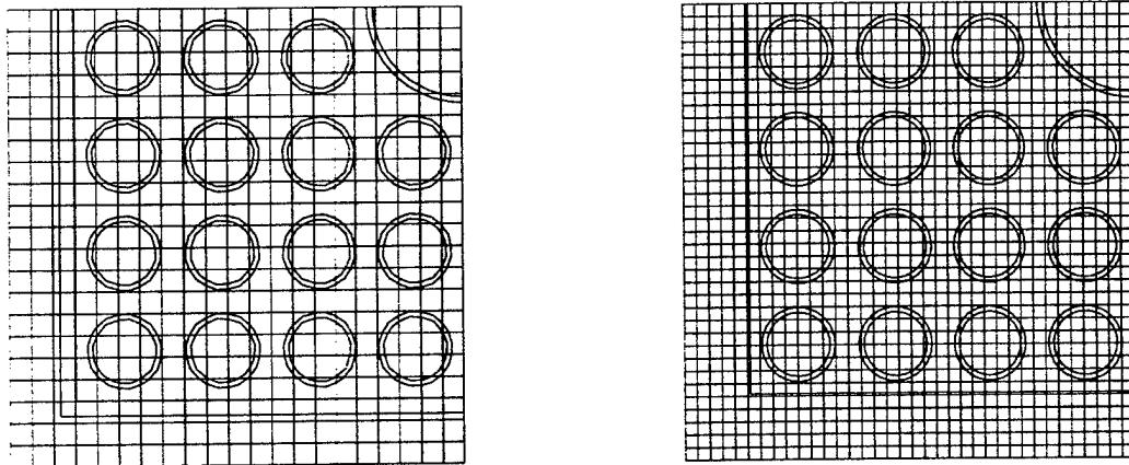
Fig. 1. NEWT 36×36 and 21×21 (nominal) grid structures with inlaid bodies.
