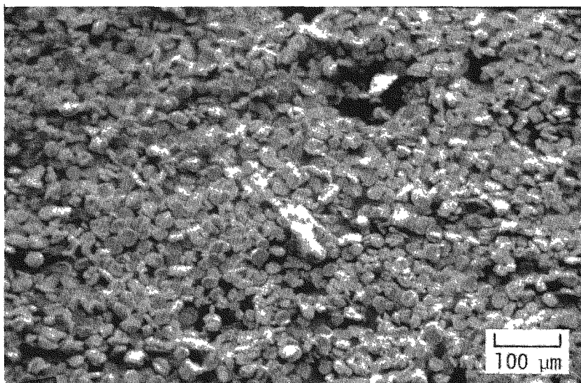
FIGURE 14. ^{239}\text{PuO}_2 Produced by Precipitation of Pu(IV) Oxalate. Up-down temperature variation. Sample T-2K.
