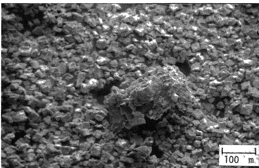
FIGURE 9. ^{239}\text{PuO}_2 Produced by Precipitation of Pu(IV) Oxalate. 150-rpm stirring during feed addition Sample T-2D.
