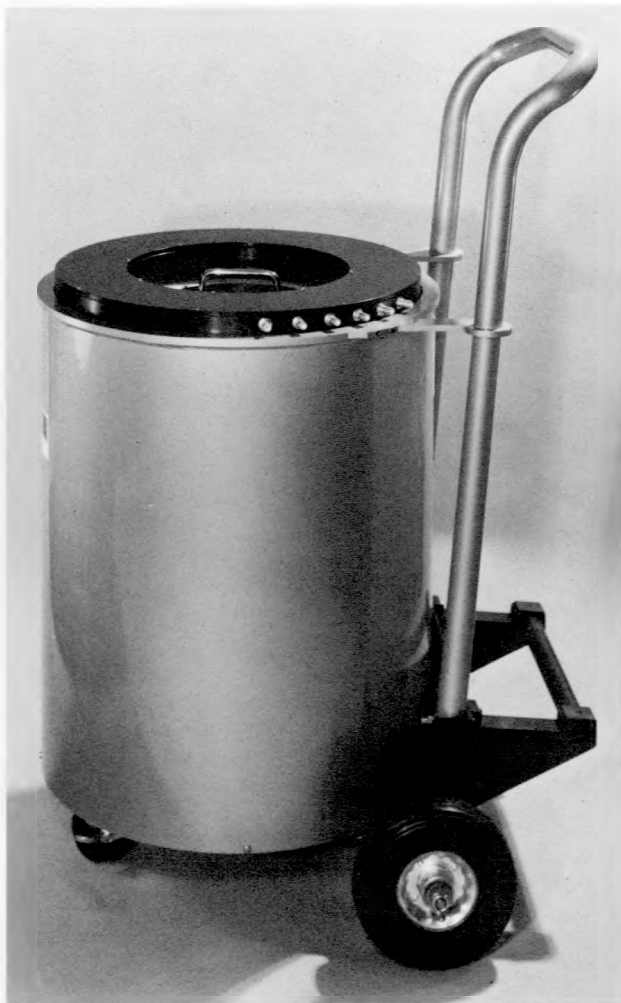
Fig. 10. Detector body and transport cart for the laboratory prototype AWCC for the assay of ^{235}\text{U} and ^{233}\text{U} .
