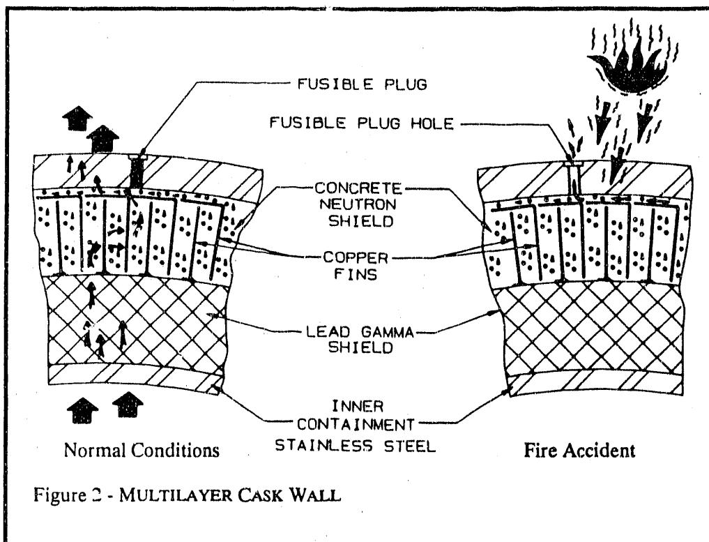
Figure 2 - MULTILAYER CASK WALL
