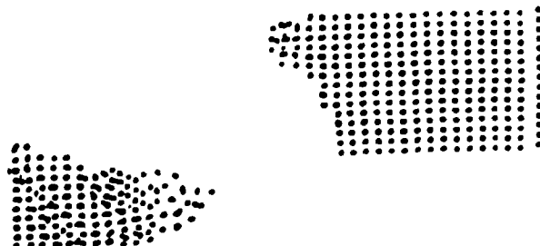
Fig. 4. Specimen B is completely broken into two pieces. Six-fold symmetrical structure is also disappeared.
