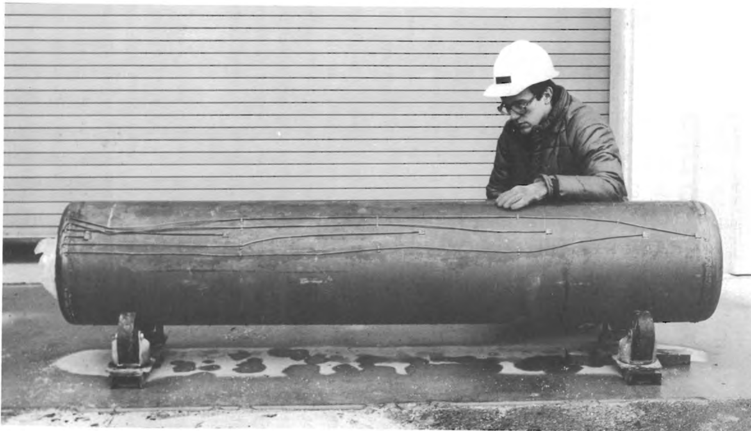
FIGURE 11. Full-Scale In-Can Encapsulation of Marbles in Lead
