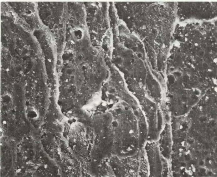
Figure 3-6. Series of Micrographs Showing the Progressively Heavier Deposits on Fin Surface by Deposits on Nearing a Heated Tube
