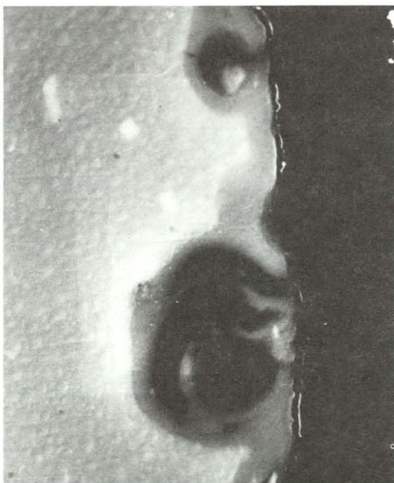
Figure 3-9. Micrograph of a Cross Section of a HOTERV Aluminum Heat Exchanger Fin After ~300 Cycles of CDL Testing
