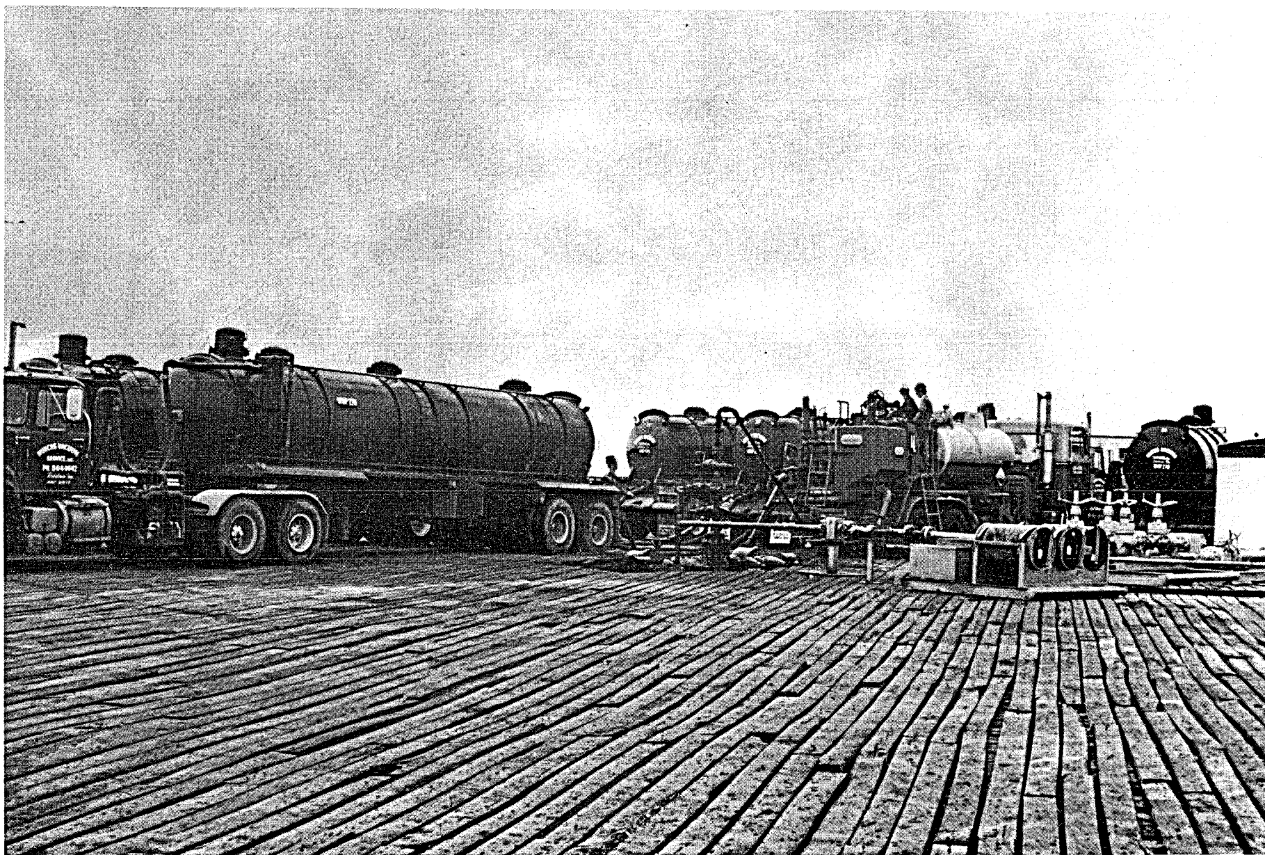
Photo 10-1 20,000-gallon acid job in progress. Acid is being injected down the tubing.
