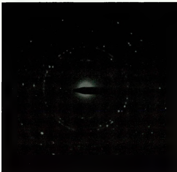
Fig. 15. SAD from fine-grain oxide on Fe-25Cr, 1 atm. O_2 , 700°C, 4h; oxide is Cr_2O_3 .
