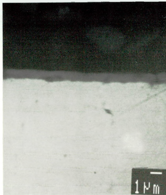
(b) Fe-25Cr-1Ce; X-Section (BEI)
