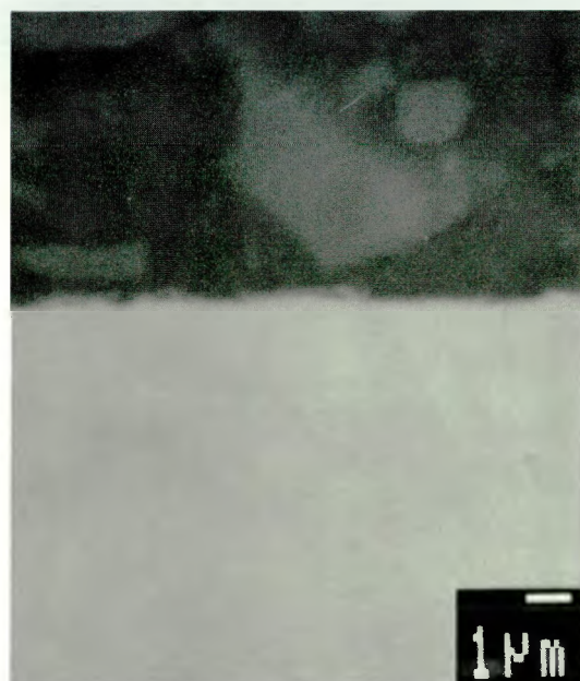
(r) X-section, Fe-25Cr-6Al-0.3Hf, HR (BEI)
