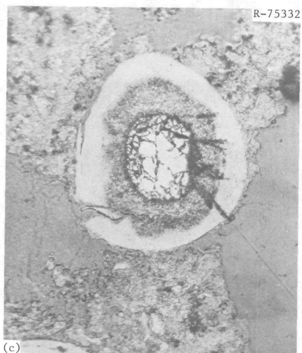
Fig. 10.6. Effects of Iron Contamination. 250 \times . Triso UC 2 fissile particle from RTE-2-6-1-1 (a) under bright field and (b) under polarized light. (c) Biso ThC 2 particle from RTE-2-6-1-1 under bright field. Reduced 16.5%.
