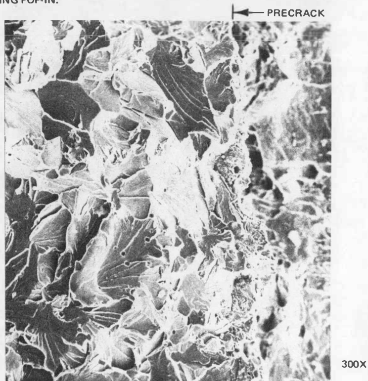
D. SPECIMEN G14 (TREATMENT E), CTS, SHOWING FATIGUE PRECRACK (RIGHT) AND QUASI-CLEAVAGE (LEFT) CHARACTERIZING BRITTLE POP-IN. DIFFERENCE IN ELEVATION BETWEEN PRECRACK AND QUASI-CLEAVAGE ZONES INDICATES CRACK OPENING STRETCH PRIOR TO CRACK GROWTH.
