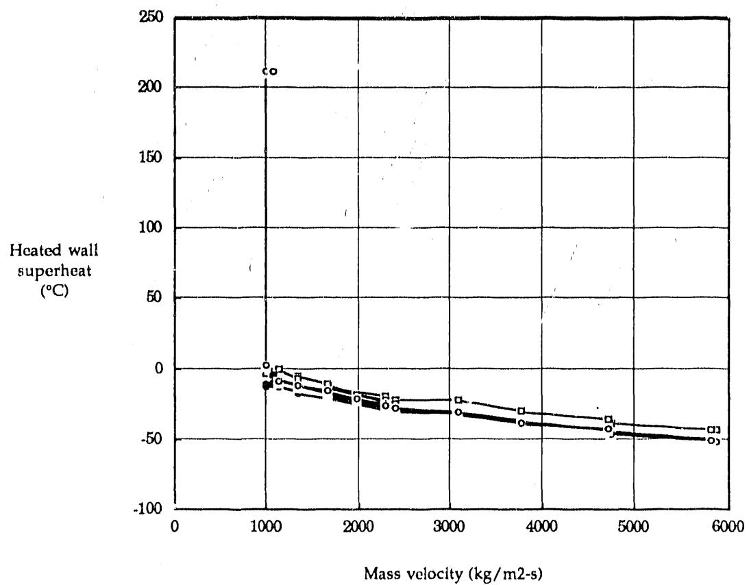
Figure 6. Variation of channel outlet wall superheat with mass velocity. All four channels shown; northwest channel is hot. Average heat flux  $360 \text{ kW}/\text{m}^2$ . Inlet temperature  $105^{\circ}\text{C}$ . Exit pressure  $352 \text{ kPa}$ .
