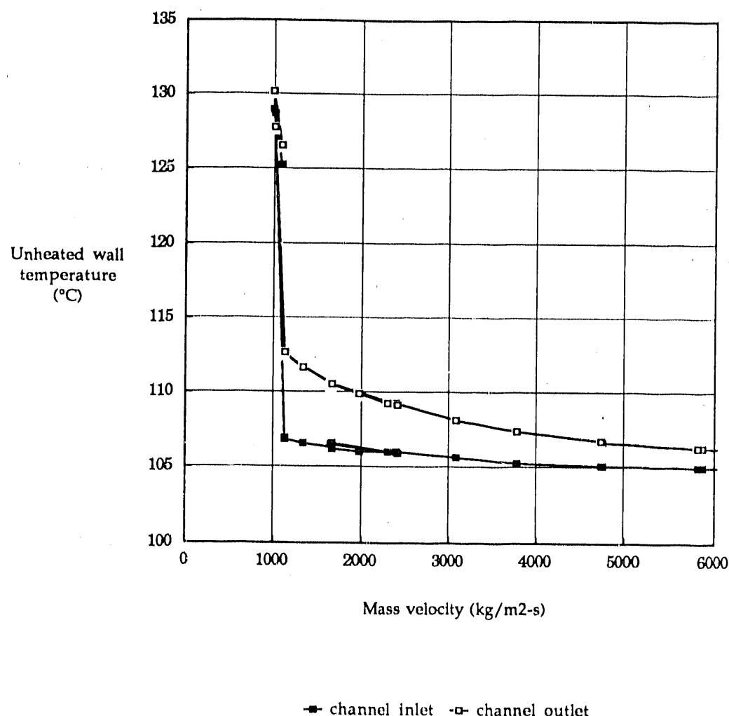
Figure 5. Variation of unheated wall temperature with mass velocity. Data from northwest channel. Average heat flux 360 kW/m<sup>2</sup>. Inlet temperature 105°C. Exit pressure 352 kPa.
