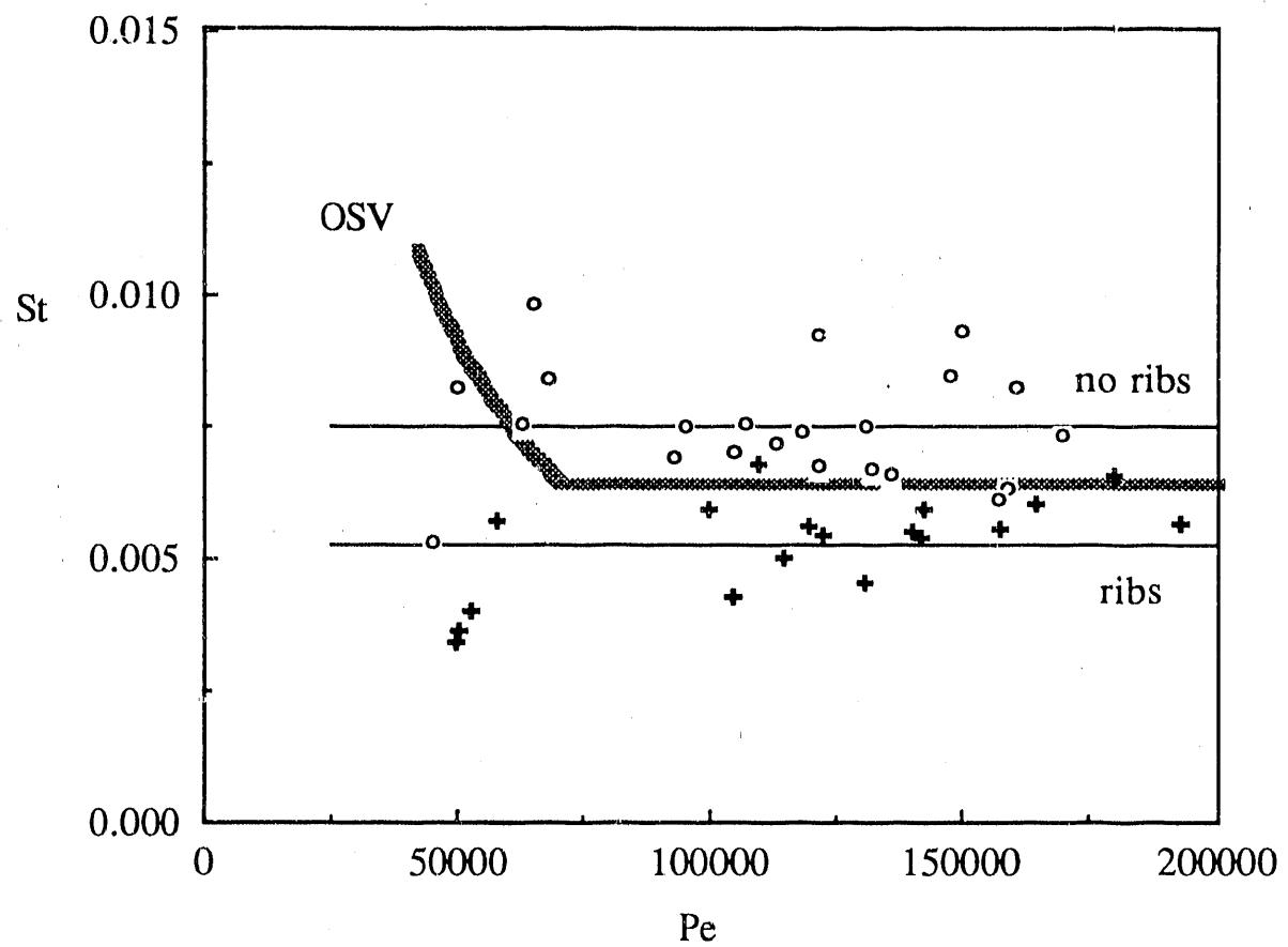
Figure 3. Minima of demand curves for heated test section, with and without ribs. Conditions at minimum expressed as Stanton and Peclet numbers and compared with the OSV correlation of Saha and Zuber (1974).
