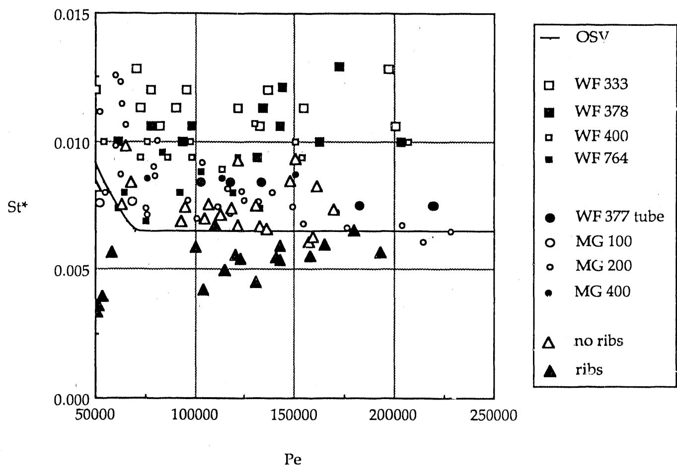
Figure 4. Minima of demand curves from several geometries and heated/flow area ratios.
