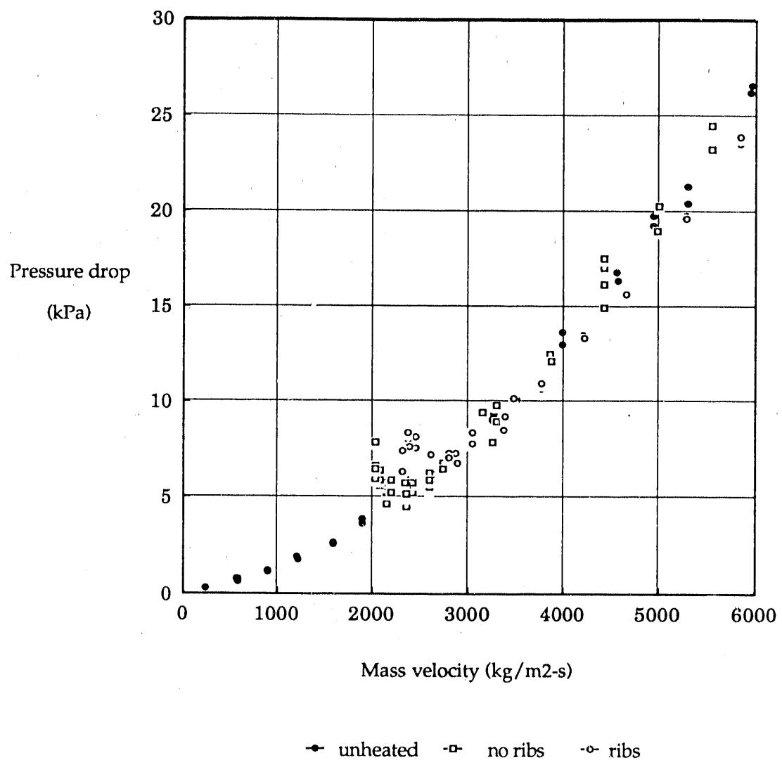
Figure 2. Demand curves for test section, with and without ribs. In heated tests, average heat flux 1.10 MW/m<sup>2</sup>. Inlet temperature 105°C. Exit pressure 331 kPa.
