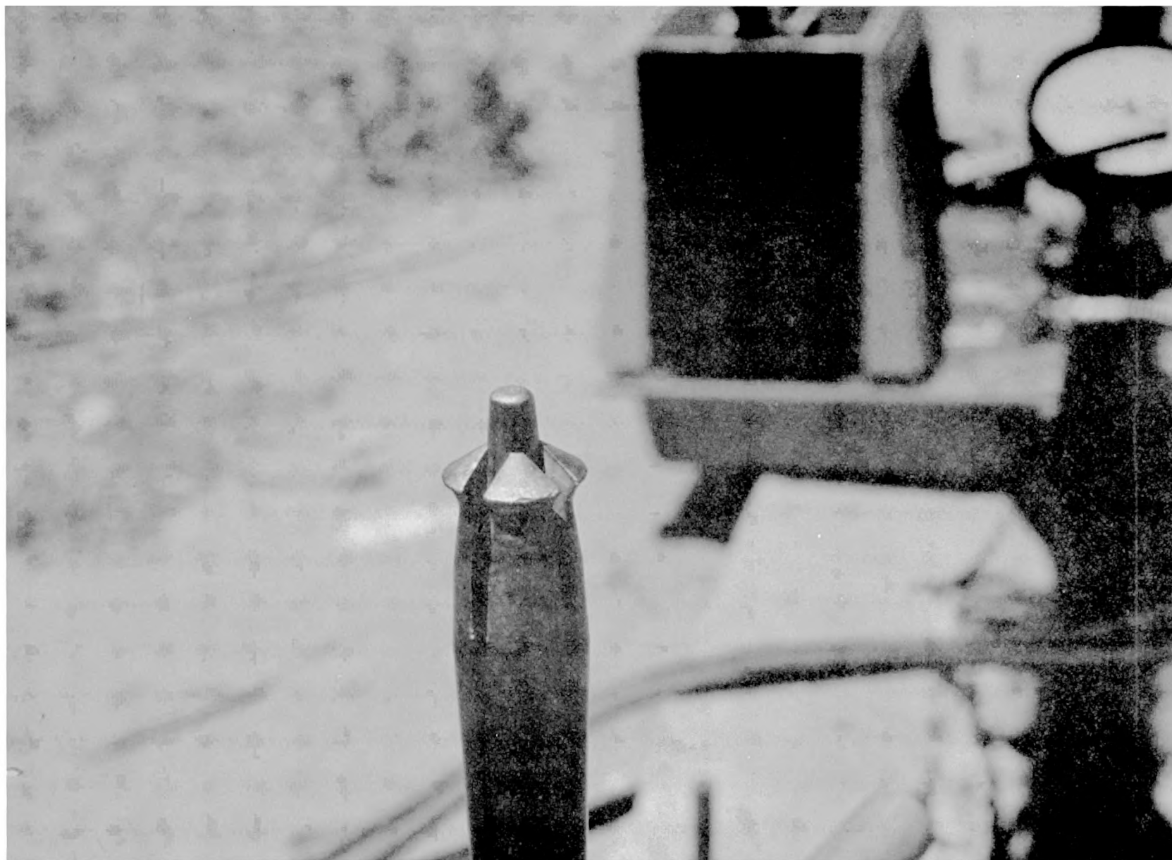
FIGURE 20. Expanding Bit Used in Concrete Spalling Technique
