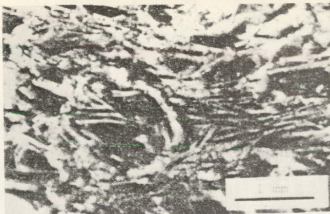
Fig. 5.5 Microstructure of the As-solidified Reactants Found in the \beta -alumina Tube at Level 8.3 cm.
