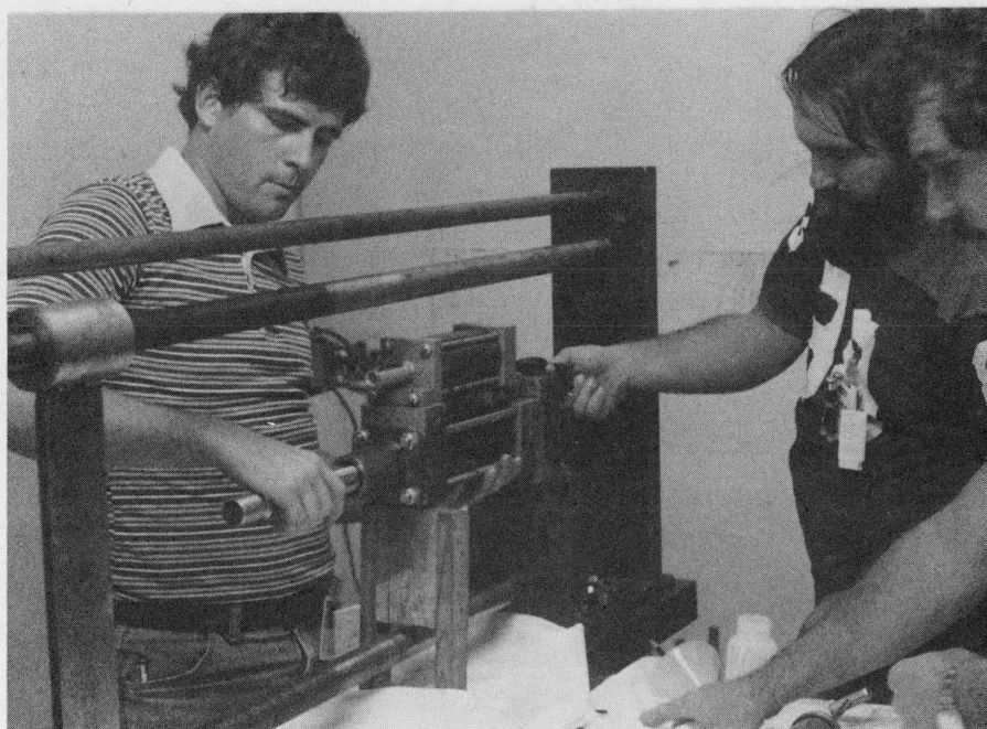
Figure 219. Placing Hydraulic Snubber in Test Stand (Browns Ferry)
