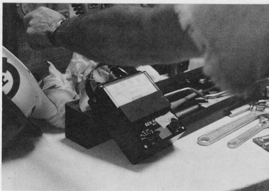
Figure 221. Voltmeter being Used as a Tachometer (Browns Ferry)
