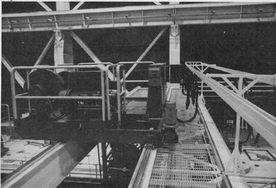
Figure 23. Bridge Trolley Drive Motor and Upper Cab Support Equipment Main Hoist (Browns Ferry)
