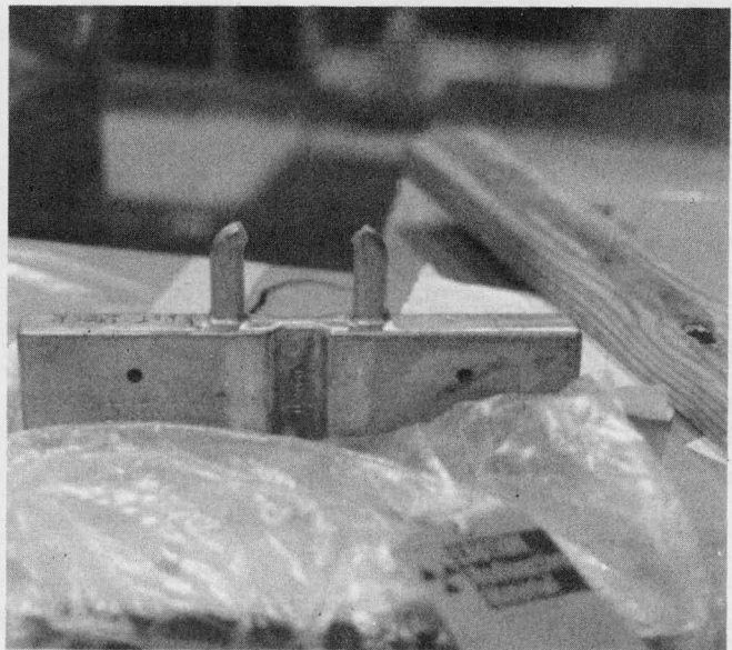
Figure 125. Aluminum Blade Guide Bracket (Fitzpatrick)
