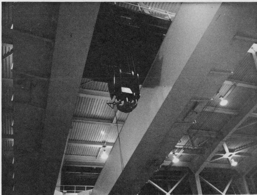
Figure 25. Refueling Floor Overhead Crane with Twenty-Ton Hoist and Dual Hook (Browns Ferry)
