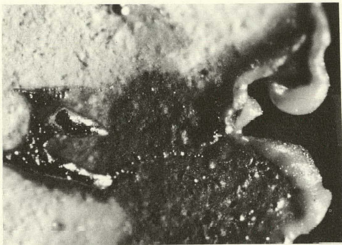
Figure 4. Part of a vapor-grown oxide cell after passing high polarization currents. The rounded edges of the oxide and beads of platinum indicate melting had occurred.
